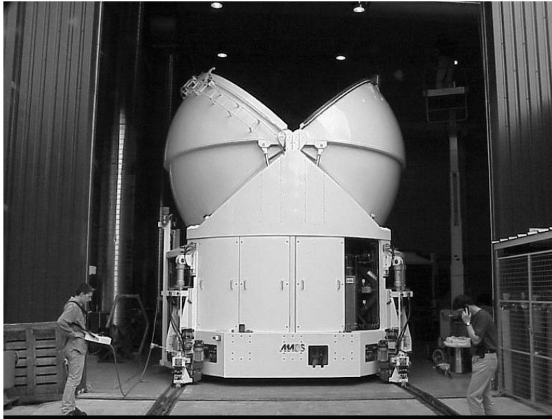
Figure 4. The first Auxiliary Telescope (AT) during final integration at AMOS in Belgium. The 1.8 m telescope with Alt-Az mount like the Unit Telescopes provides a collimated beam 1.2 m underground that is sent towards the Delay Line Tunnel through insulated light ducts. The ATs are relocatable on 30 stations using special transporters moving on rails.
