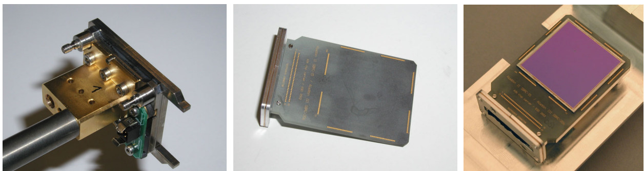
Figure 2 Pictures of the invar baseplate with the copperblock, the 8 layer AlN ceramics and the final mounted Aladdin device
