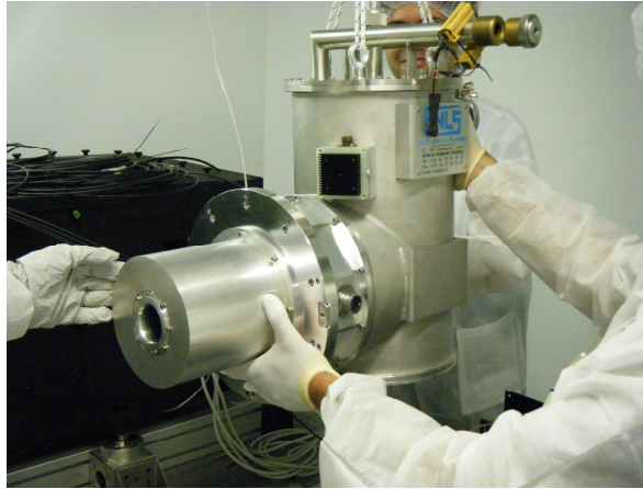
Figure 2. Photo of the dewar. Note the large distance between the window and the detector, which is roughly at the location of the widest flange.
