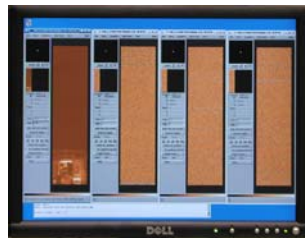
Figure 4. Four Real Time Displays visualize simultaneously the incoming data. Each display shows a group of four detectors.
