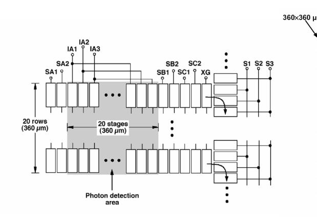
Functional drawing of a unit cell, with an integration area made of 20 x 20 pixels, each 18 µm square. These unit cells form an imaging area (IA) of 360 by 360 µm for each subaperture. These pixels are binned by rows into the storage areas SA and SB. The storage areas are small compared to the imaging area, being only one pixel wide.
