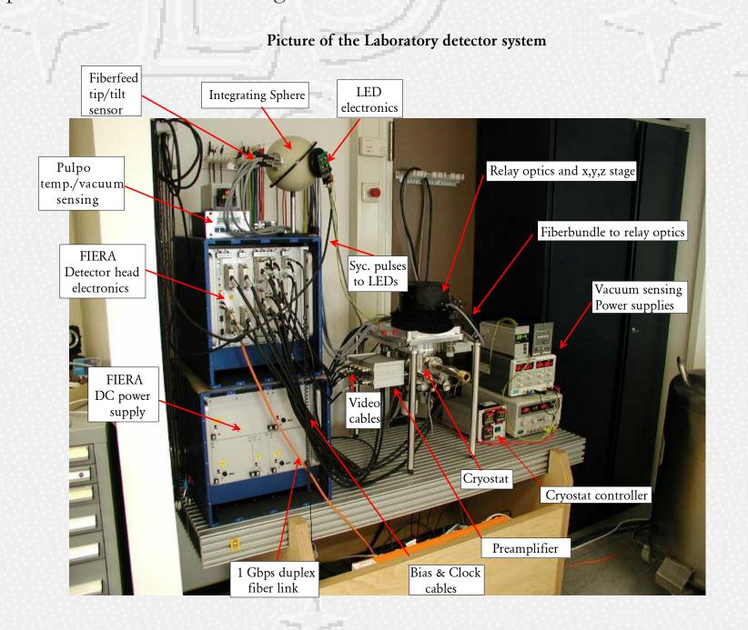
A readout noise of less than 1.5 electrons was achieved for all readout ports including the tip/tilt sensor at a readout speed of 4000 frames per second. With all pixels per per readout port binned into 12 superpixels, it was possible to read the serial register relatively slowly at 50 kilopixels per The plot shows readout noise and conversion factor versus
