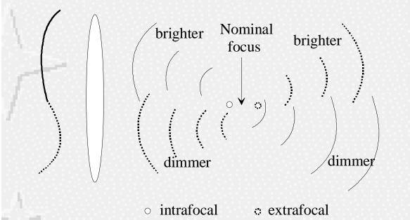
Curvature wavefront sensing looks at intensity between pupi image and image plane. Curved wavefront comes to focus before and after nominal focal plane and thus is brighter or dimmer in out-of-focus image. Must sense on both sides of focus to calibrate scintillation.
