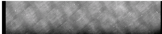
Figure 22a - 2048x512 pixel subframe of the EEV devices, one hour exposure dark frame, just after a flat field, the dark current is 43e-/pixel/hour and the "dark current" is related to the "blue diamond" pattern.
