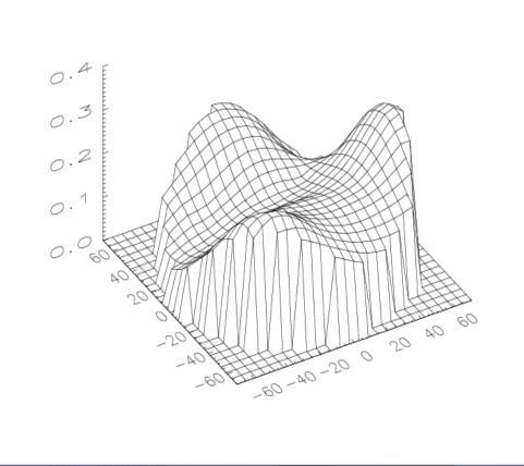
"Hole" in the middle is mostly due to the turbulent layers between deformable mirrors
