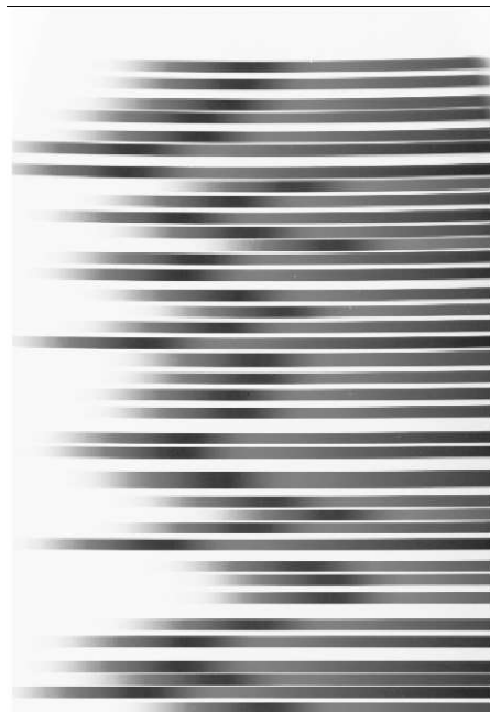
Fig. 2. Example of spatial curvature for a raw FORS2 MXU flat field.
