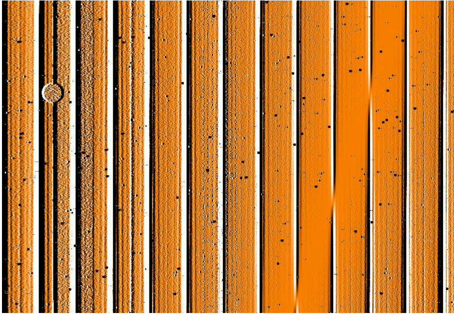
Fig. 3. Difference between a raw fiber exposure and the same fiber exposure corrected for optical distortion. Note that the fiber image is chopped in 32 slitlets and projected side by side on the detector by the image slicer.
