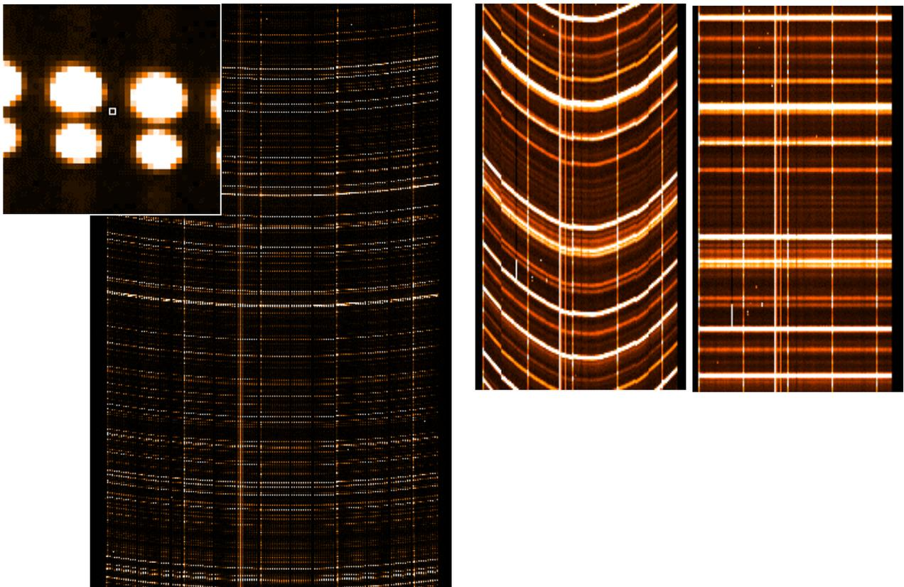
Figure 3. a. Raw arc-lamp exposure (Medusa mode), with curved spectral format. b. Product after extraction (the curvature is still present). c. Rebinned arc-lamp spectrum, with strictly horizontal emission lines.
