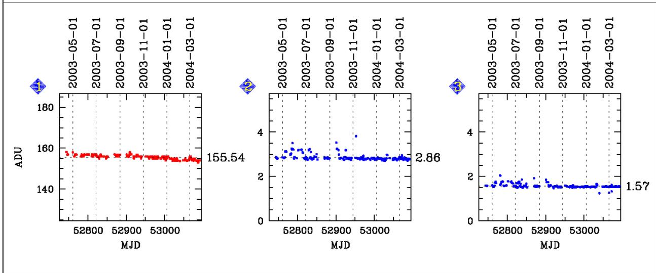
Figure 7. The behaviour of GIRAFFE bias level (item 1), RON (raw frame; item 2) and RON (master frame, item 3) during the first year of operation. The master bias is usually made of 5 input raw frames. Numbers at the right side are mean values over the range of time.
