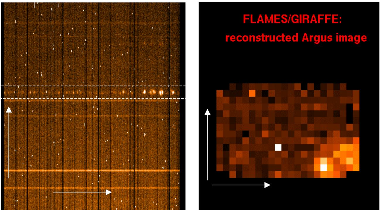
Figure 5. Image reconstruction of GIRAFFE Argus spectra. a. The reduced Argus spectrum, same format as Figure 4b. The two white lines mark a spectral range which defines the extraction limits for the reconstructed image. b. Reconstructed Argus image in the wavelength range defined in a. The extracted signal is rearranged in (arbitrary) X and Y coordinates on the sky.
