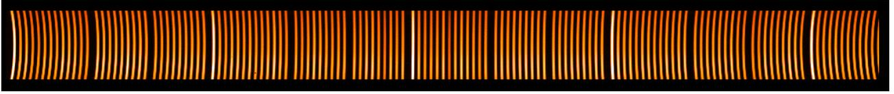
Figure 2. GIRAFFE Flat field data. a. Raw flat field. The five bright fibres are the SIMCAL fibres. The vertical scale is highly compressed.
