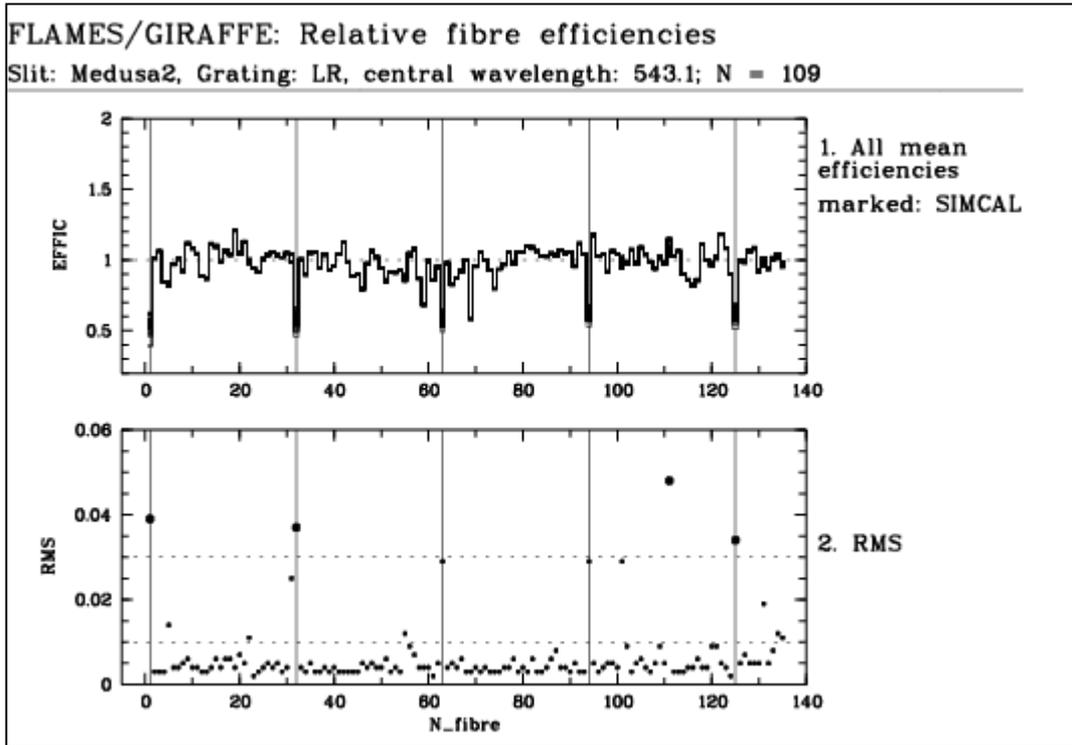
Figure 9. Top: mean efficiencies, normalized to one. The fibres are illuminated by the robotic calibration lamp, except for the SIMCAL fibres which are lit by a dedicated lamp with intrinsically more unstable signal. A total of 109 measurements are plotted here on top of each other. Bottom: the rms of the variations against the mean value from top. Most fibres are stable within 0.3 %. Apart from the SIMCAL fibres, only one object fibres shows rms variations of more than 3% (upper broken line).
