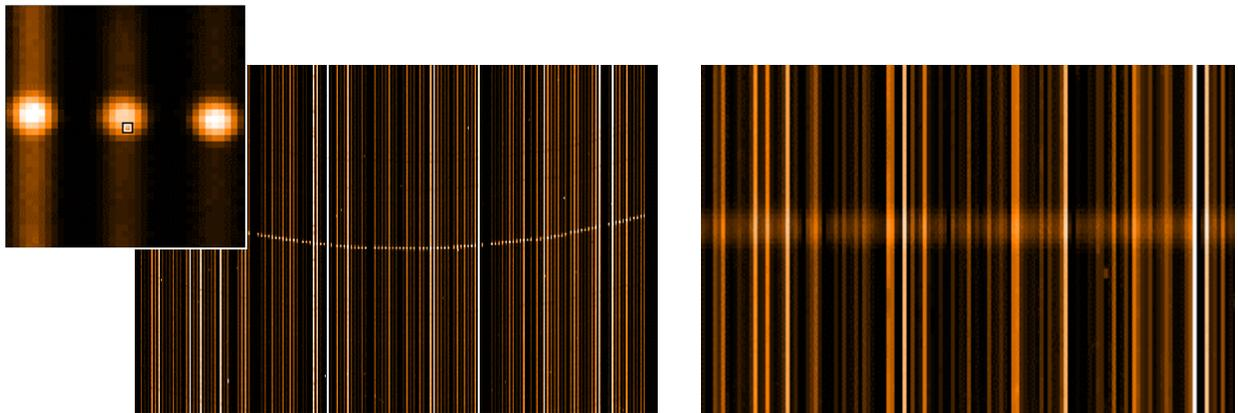
Figure 4. GIRAFFE science frame. a. Raw science frame in a Medusa mode. The dotted line is the OI 6300 Å emission line. The close-up shows that line in three adjacent fibres. b. Reduced science frame, in the region of the OI line. Each column represents a science spectrum, with wavelength increasing upwards.
