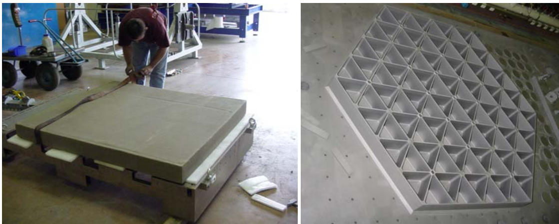
Figure 6-50. Precursor (left) and 1-m sintered SiC segment (right). Courtesy Boostec.
