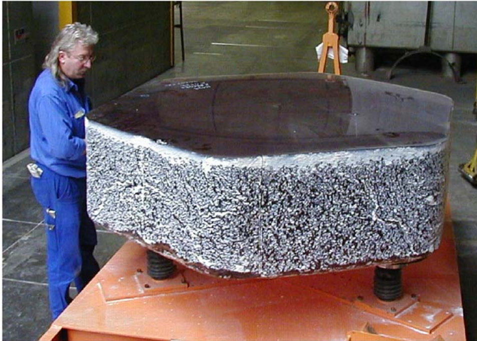
Figure 6-47. Zerodur hexagonal cast. Courtesy Schott.
