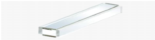
Fig. 5-28 . Light pipe made with high-efficiency mirrors. Glass rods with total internal reflection are also commonly used.
