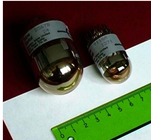
Fig.3.11. MAGIC focal-plane detector system: The camera has “pixels” of 0.1 degrees in the central section, up to 1.2° radius, and a ring of 0.2° pixels extending to 1.8° radius. The camera detectors are hemispherical photomultiplier tubes, operated at low gain in order to prevent damage from the night-sky background or during operation in moonlight.
