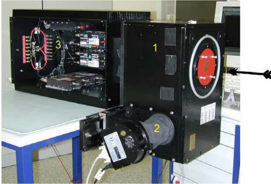
Fig.A3.17. The OPTIMA instrument with its side opened, showing locations of its photon-counting avalanche photodiodes (3). The target acquisition optics (filters, target imaging, and fiber pick-up) is located in (1), and the CCD camera is mounted externally (2). (Kanbach et al. 2003).
