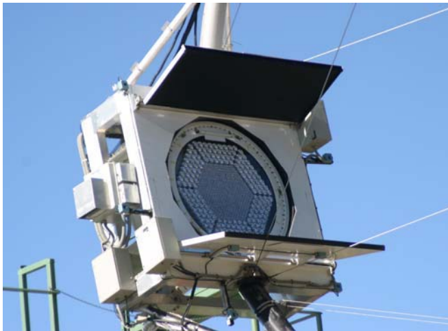
Fig.3.11. MAGIC focal-plane detector system: The camera has “pixels” of 0.1 degrees in the central section, up to 1.2° radius, and a ring of 0.2° pixels extending to 1.8° radius. The camera detectors are hemispherical photomultiplier tubes, operated at low gain in order to prevent damage from the night-sky background or during operation in moonlight.
