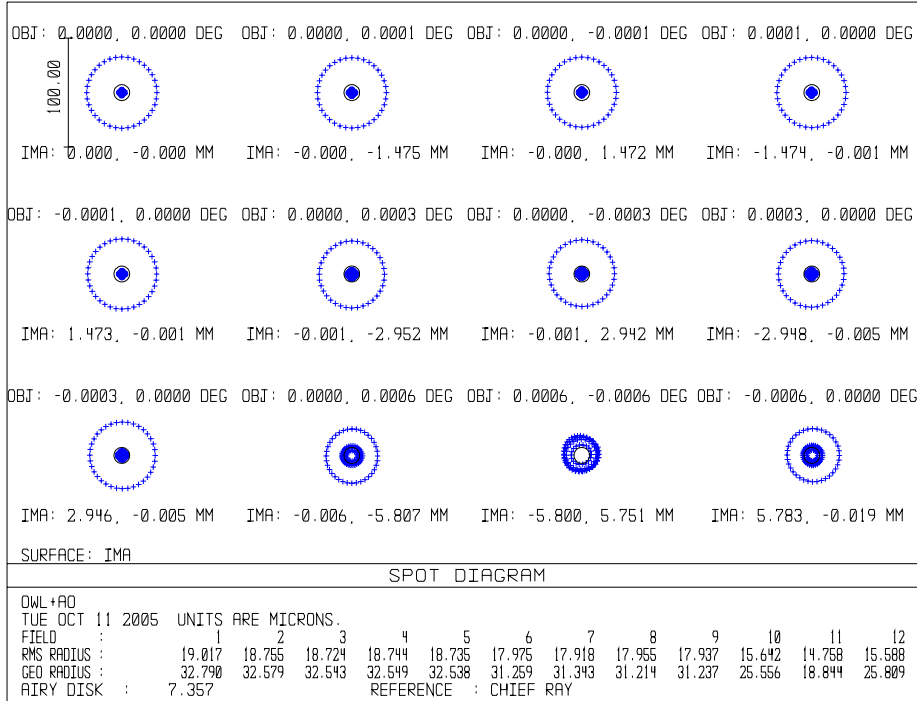
Figure 7-6: Spot diagrams for a 4 arcsec field. Wave-length is 1 micron. The field curvature is about 200 mm. Field points are 1 in the center (top left), then from left to right 4 points at corners at 0.5, at 1 arcsec separations and 3 points at 2 arcsec separations.
