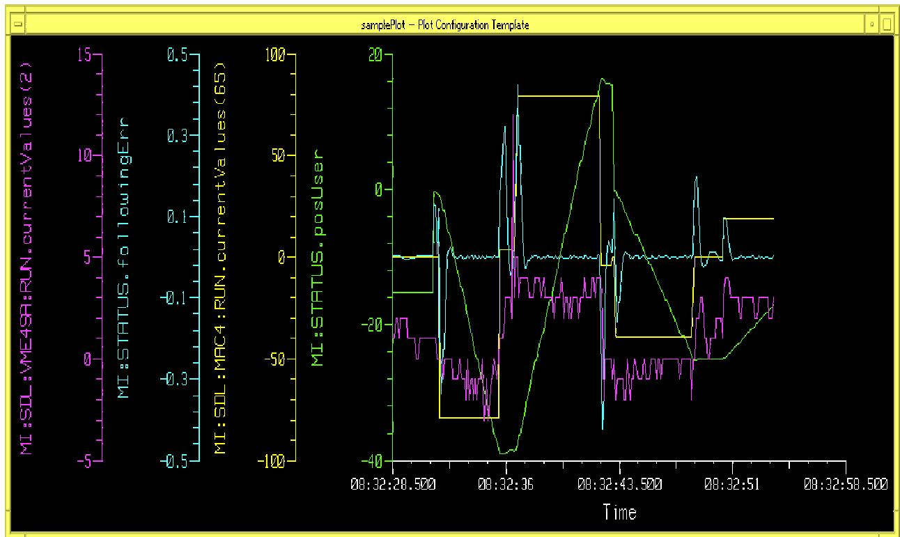
This diagram shows the time evolution of the position (mm), velocity (Enc/ms), following error (mm) and current (Dig) for a typical HW initialization sequence.
