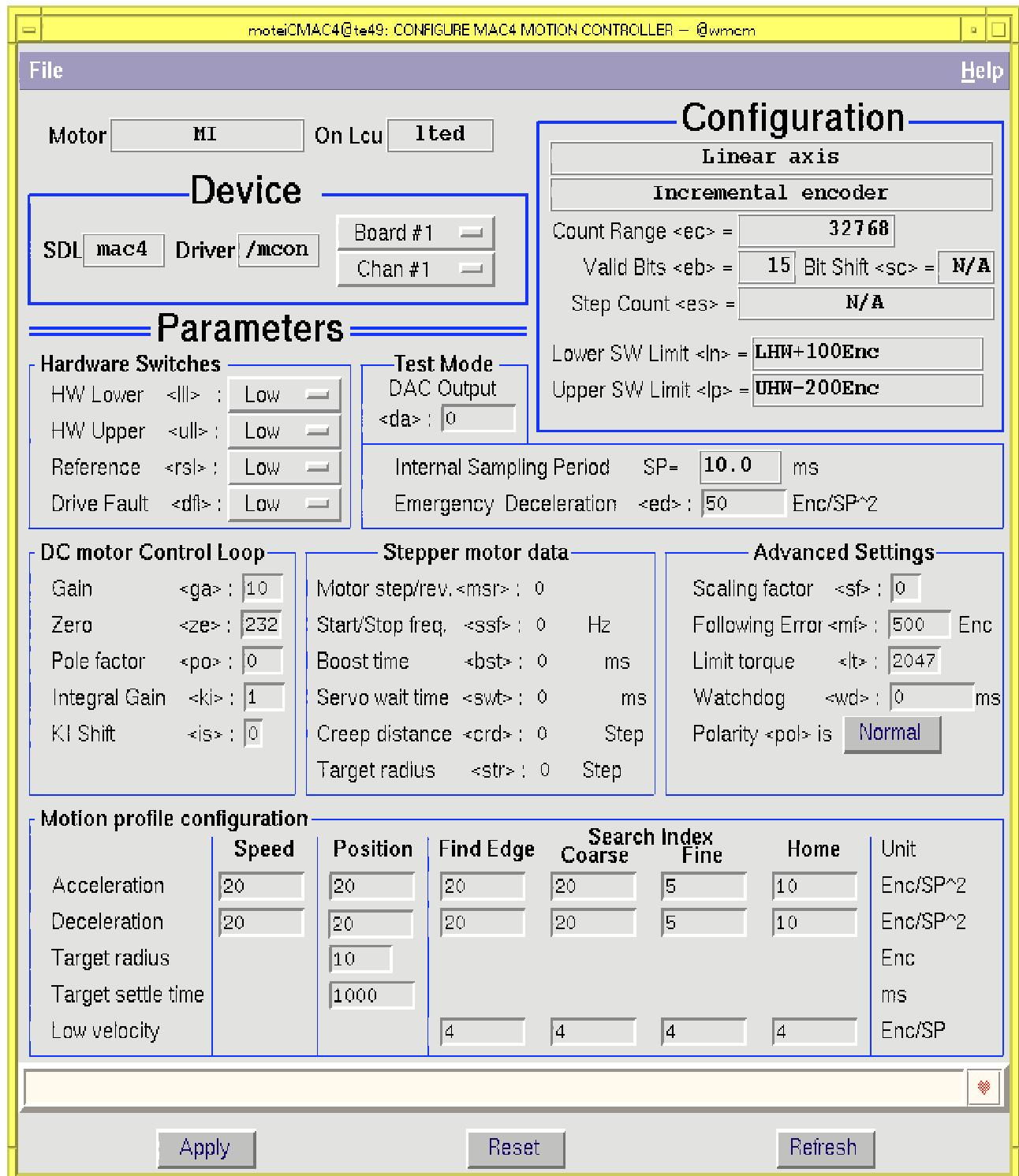
The **Device** part allows the setting of the associated hardware channel. The board selector refers to the board index with increasing base address; the channel selector refers to the outputs as labelled on the backplane and on the board front panel.
