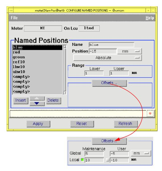
The ListBox shows the list of all defined Named Positions or <empty> if the row is available. Whenever an entry is selected (by clicking on it with the mouse), the panel is updated with the position name and its parameters. Each named position shall be described as a Nominal position and the two Lower and Upper range values that define the domain in which the name shall be valid.
