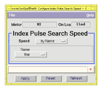
This panel is dedicated to the definition of the speed to be applied when performing the second step of the search motion to the index pulse of the encoder. See 5.2.8 for man page.
