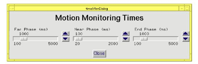
These times are defaulted to 1000, 200 and 1000ms resp. and are applied when defining the speed by value.
