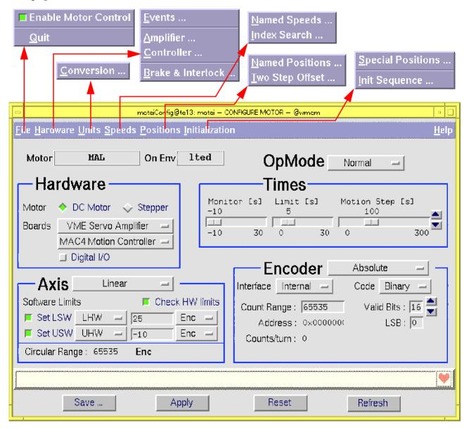
The panel is to be read from the part Hardware, down to Axis, Encoder and Times. According to the current settings, some items may not be enabled, some values may be modified as a consequence of a previous setting.
