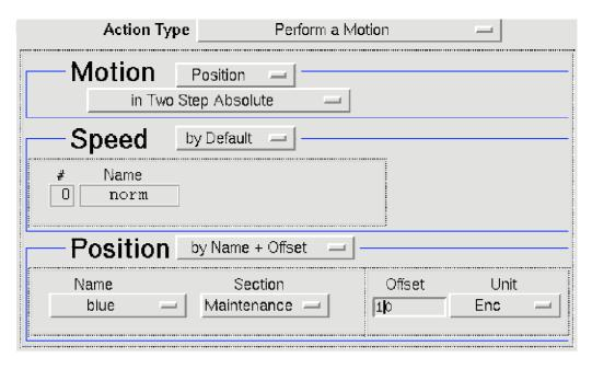
This is the main action dedicated to the description of motions. At this stage none of the special positions is known therefore care should be taken when defining the target positions when not absolute. As well, absolute positions do make sense only after the axis has been calibrated, i.e. a known position is assigned a known value (e.g. find the Reference Switch and calibrate the position as 0 Enc).
