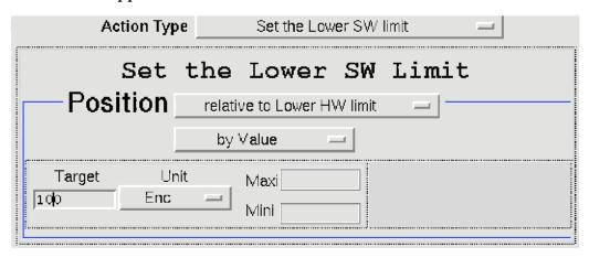
Only on Linear Axis, this setting are overridden by the SW limit settings as of the Main Configuration panel (see 3.4).
