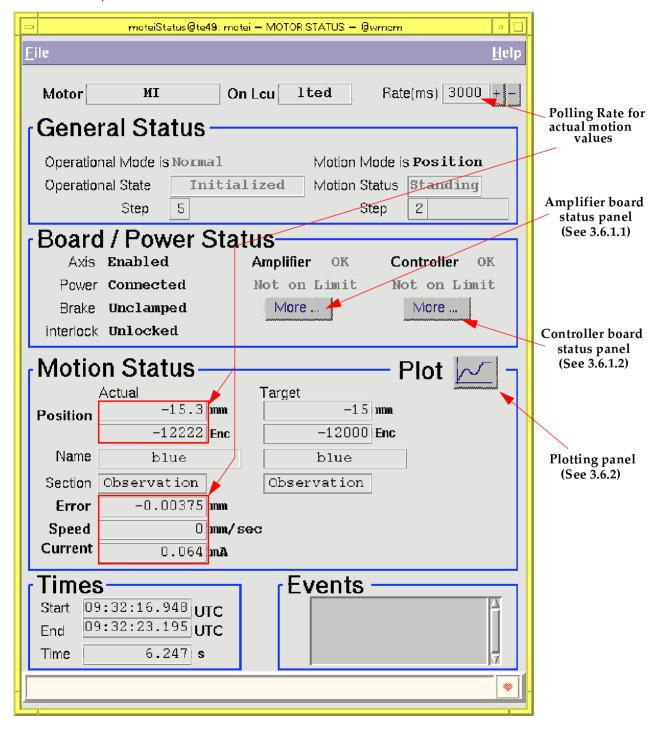
It is divided into five parts: from top to bottom, **General**, **Board/Power**, **Motion**, **Time** and **Events Status**. The information displayed is assumed to be self-explicative. The **Position** information displays both **Actual** and **Target** position in **User** and **Encoder** units.
