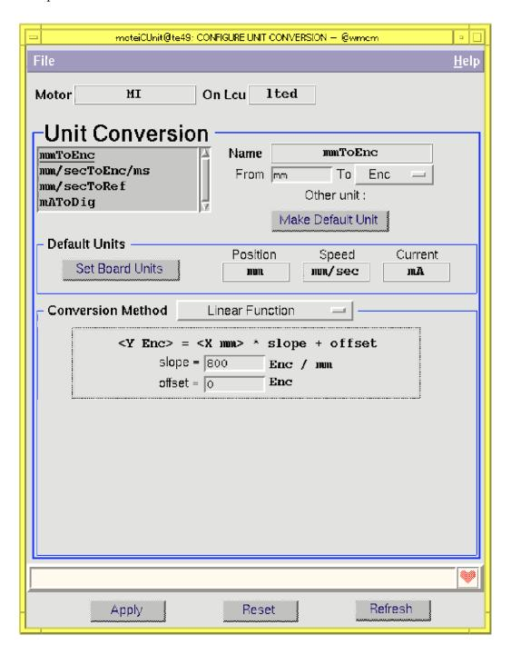
The panel shown above displays the default set of units and the table of unit conversion methods of the selected motor, see 5.2.6 for man page. The listBox displays the names of the conversion method or <empty> if the row is available. Whenever a method is selected (by clicking on it with the mouse) the panel is updated with the source unit, target unit, conversion method and its related parameters as from the database.
