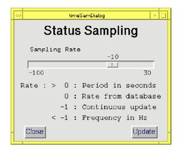
Note: High sampling rate implies also a higher CPU load. In the standard HW configuration MCM needs approx. 9.5ms to refresh the status. When many motors are controlled in parallel, high rates may not be effective.
