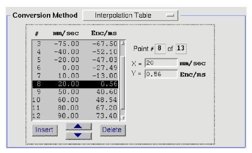
Minimum 2 points, function must be monotonous Edges of conversion domain must be included
