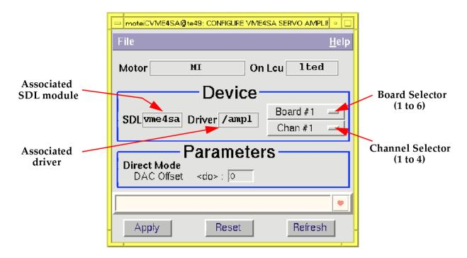
The **Device** part allows the setting of the associated hardware channel. The board selector refers to the board index with increasing base address; the channel selector refers to the outputs as labelled on the backplane and on the board front panel.
