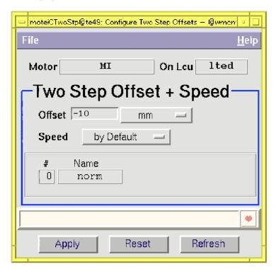
The offset is a relative value which will be added to the target position value so as to define the position to move to during the first step:
