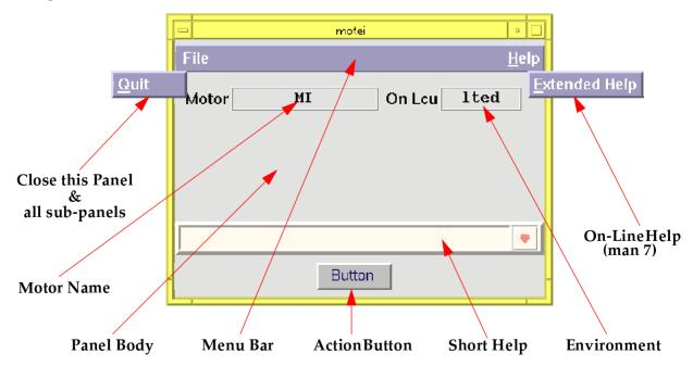
Each panel contains a menu bar, a short help field, action buttons and 2 output fields that show the selected motor and the working environment. The panel body contains all UIF elements needed by the dedicated function of the panel.
