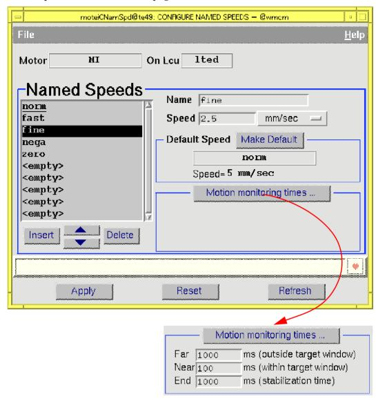
The ListBox shows the list of all defined Named Speeds or <empty> if the row is available. Whenever an entry is selected (by clicking on it with the mouse), the panel is updated with the speed name and its parameters. The default speed is also displayed and it is possible to set its value by pressing the Make Default button, the settings currently present in the panel will be used.
