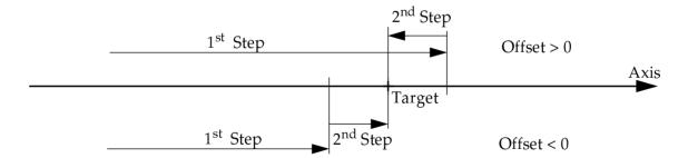
This type of motion is meant to correct for eventual mechanical backlash, and thus increase the precision of the positioning.
