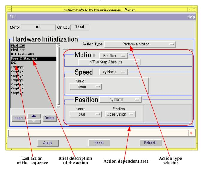
The ListBox shows the list of all defined Actions or <empty> if the row is available. Whenever an entry is selected (by clicking on it with the mouse), the panel is updated with the action type and its parameters.
