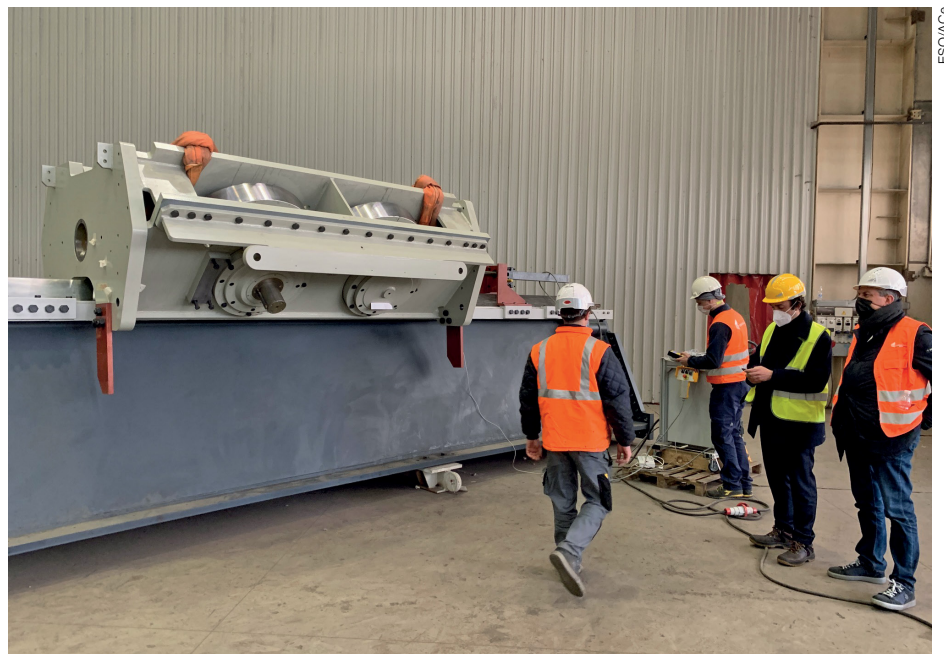
Full-scale functional testing of one of the 36 ELT dome rotation trolleys at Cimolai facility (Italy).
