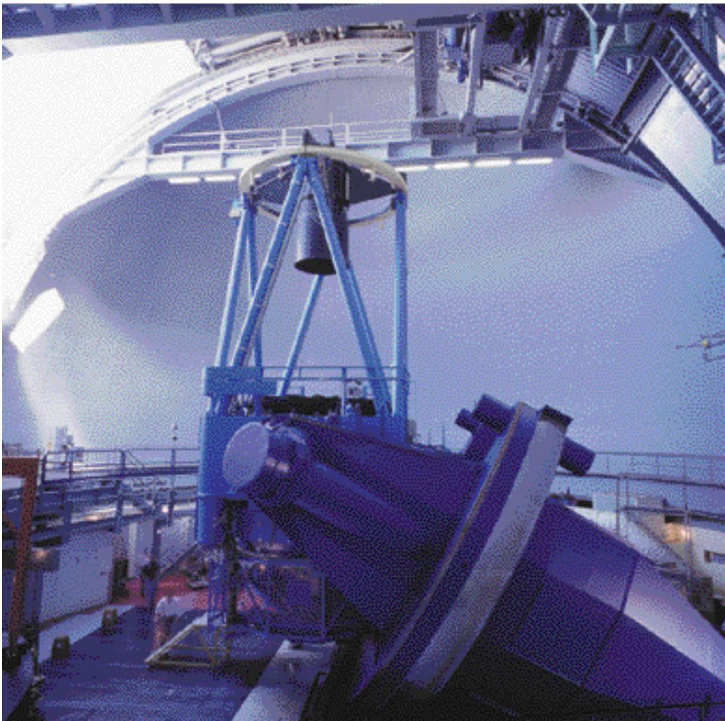
The 3.6-m telescope after installation of the re-aluminised M1.
