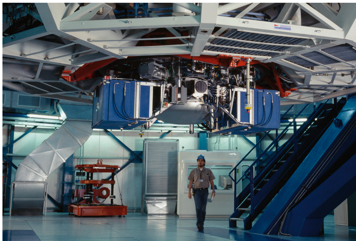
The VLT spectrometer and imager for the mid-infrared (VISIR) mounted at the Cassegrain focus of UT3.
