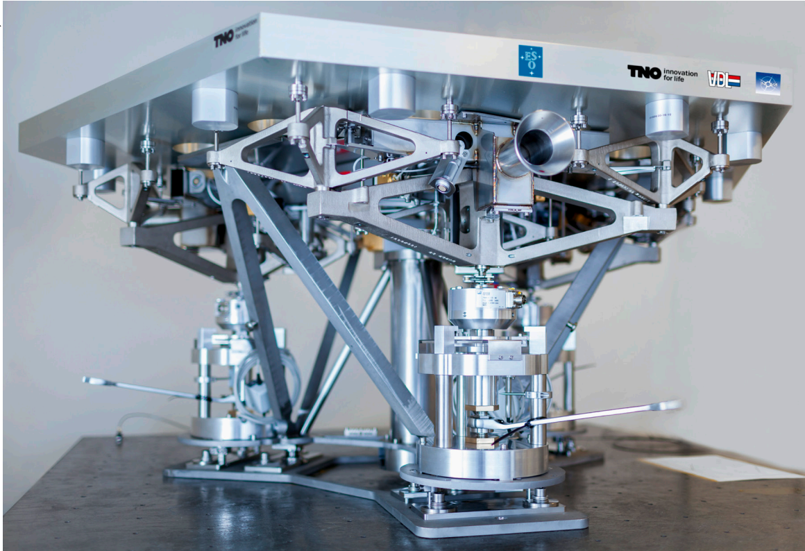
Figure 2. One segment support structure of the giant primary mirror of the ELT undergoing testing.
