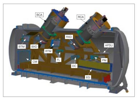
Figure 4. Opto-mechanical drawing of the ESPRESSO spectrograph is shown. Key to components: APSU: Anamorphic Pupil Slicer Unit; BCA: Blue Camera; BTM: Blue Transfer Mirror; BXD: Blue
