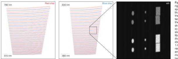
Figure 2. Shown left to right: Format of the red spectrum: format of the blue spectrum; zoom of the pseudo slit. This latter shows the image of the target (bottom) and sky fibre (top). Each fibre is re-imaged into two slices. The three sets of fibres, corresponding (from left to right) to the standard resolution 1-UT mode, ultra-high resolution 1-UT mode, and mid-resolution 4-UT mode, are shown simultaneously.
