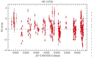
Figure 11. Ten years of RVs for Tau Ceti are plotted as measured by HARPS. The overall dispersion is 1 m s<sup>-1</sup>. Timebinning of the data reduces the dispersion as expected with the square root of the number of observations down to 20 cm s<sup>-1</sup>. Most important yet, is the absence of any longterm trend, thus proving the exquisite precision of HARPS.
