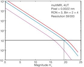
Figure 9. Achievable signal-to-noise ratio (SNR) plotted as a function of stellar visible magnitude for the singleHR (left) and the multiMR (right) modes. Red, blue and magenta curves indicate exposure times of 3600 s, 1200 s and 60 s, respectively.
