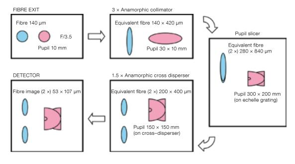
Figure 3. Conceptual description of pupil and fibre image at relevant locations of the ESPRESSO spectrograph.
