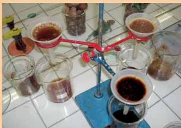
Figure 5: Filtering the water and crushed gall mixture
