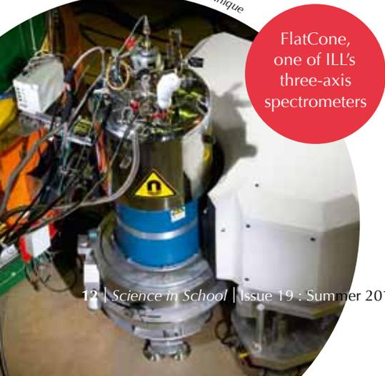
FlatCone, one of ILL's three-axis spectrometers
