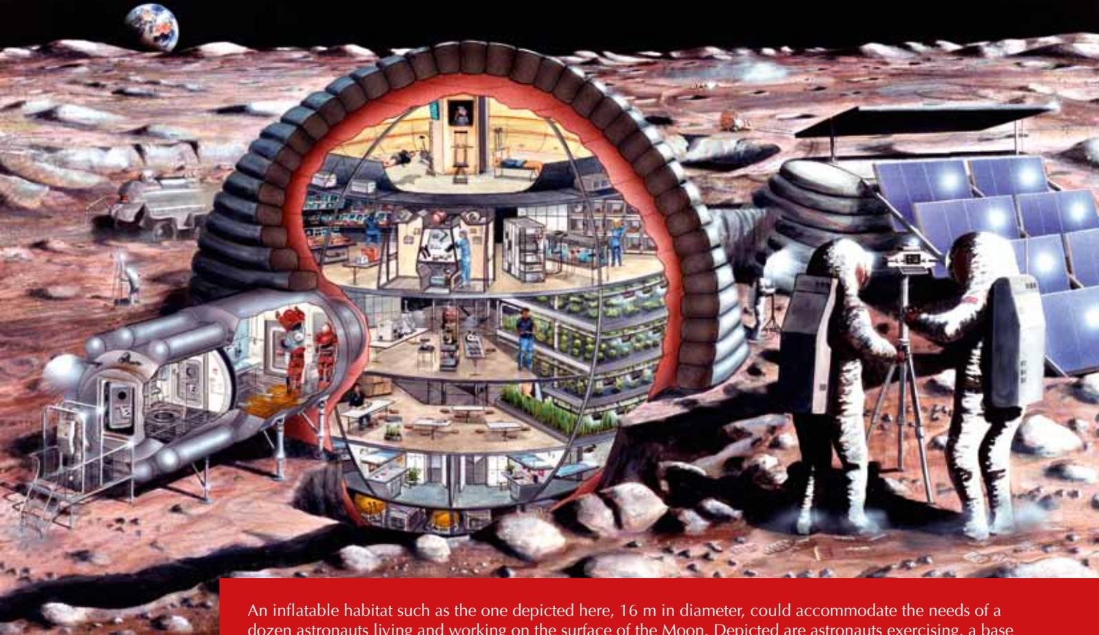
An inflatable habitat such as the one depicted here, 16 m in diameter, could accommodate the needs of a dozen astronauts living and working on the surface of the Moon. Depicted are astronauts exercising, a base operations centre, a pressurised lunar rover, a small clean room, a fully equipped life sciences lab, a lunar lander, selenological (lunar geology) work, hydroponic gardens, a wardroom, private crew quarters, dust-removing devices for lunar surface work and an airlock
