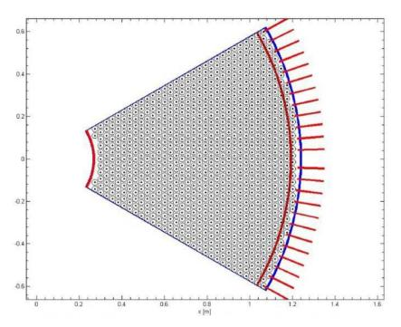
Fig. 3: Mirror shell layout with actuator pattern
