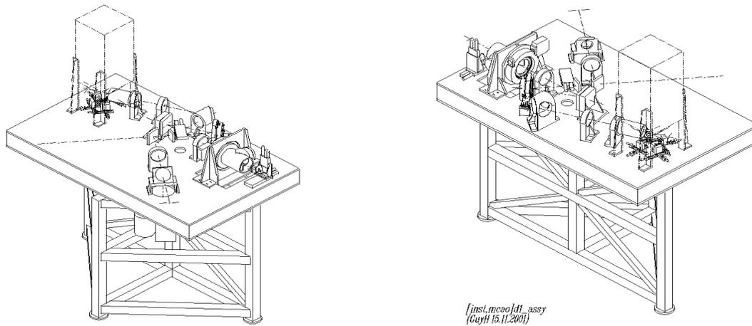
**Figure 2.** Mechanical design concept of the MAD bench. The elongated box above the bench represents the LOWFS volume. The Multi Shack–Hartmann WFS is located below the LOWFS.
