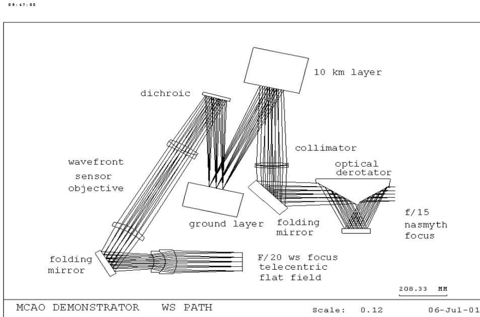
**Figure 1.** Optical design concept for MAD. The two boxes represent the two Deformable Mirrors conjugated at 0 and  $\sim 10$  Km. The IR camera is placed behind the dichroic.
