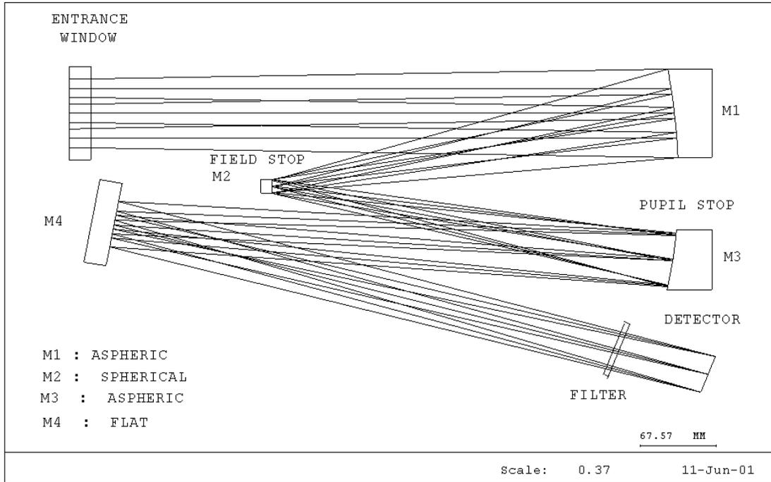
**Figure 5.** Optical design concept of the IR camera CAMCAO. The camera has diffraction limited imaging capabilities above  $1.0\mu\text{m}$  wavelength.
