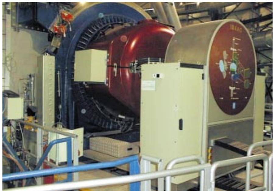
Figure 1: ISAAC installed at the Nasmyth B focus of the VLT UT1. The instrument, enclosed in its protective red cover, is attached to the adapter/rotator system at the left and has a total weight of around 1.5 tons. The box at the left contains some of the electronics required for controlling and reading the two infrared array detectors. To the right is the co-rotator system that transfers all the electrical cables and gas hoses for the closed-cycle coolers to the instrument and rotates with it and the adapter. At each side of the co-rotator are cabinets containing electronics for controlling and monitoring the instrument functions and the vacuum and cryogenic system. At the bottom can be seen part of the platform to which the instrument is attached for installation, removal and maintenance activities.
