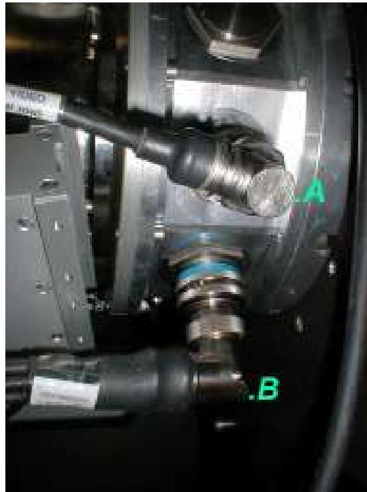
Figure 1.8: Clock and video connection on D-Marc head.
