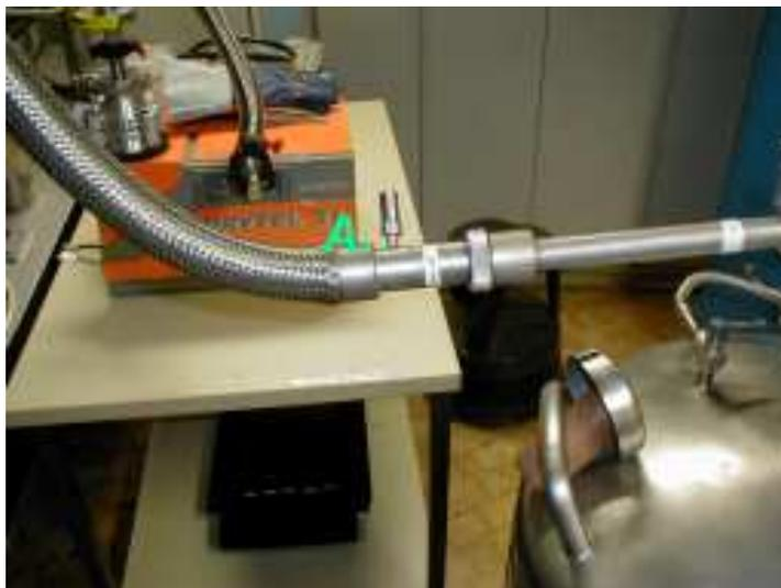
Figure 1.12: Good position of the nitrogen tube, take the valve on the tube as mark.
