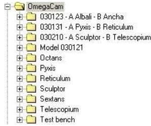
Figure 2.1: Before starting a new data acquisition, Directories need to be created. You have here for example the three directories concerning the CCD Pyxis and Reticulum. These directories 'Pyxis', 'Reticulum' and '030131 - A Pyxis - B Reticulum' are a simple copy of 'Model 030121' directory.
