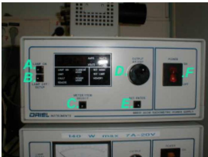
Figure 1.24: Control panel of the halogen lamp.
