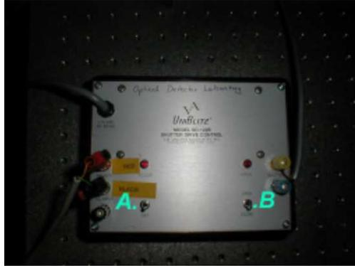
Figure 1.3: The monochromator shutter controller. Power button of the shutter (A.) and the open/close button of the shutter (B.)
