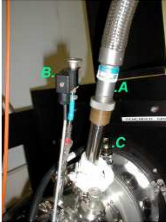
Figure 1.5: Nitrogen tube (.A), nitrogen valve (B.) and pulpo cable (.C) connected to the D-Marc head.
