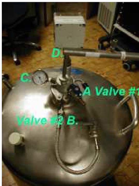
Figure 1.11: The two valves (.A and B.), valve #1 open and valve #2 close, the pressure jaugue (C.) and the extraction tube (D.) on the nitrogen bottle.
