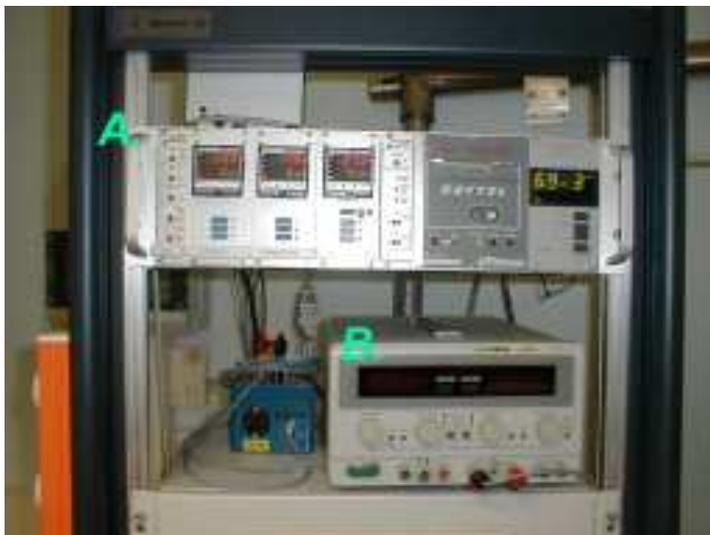
Figure 1.13: The CFC controller (A.) and the SESO power supply (B.).
