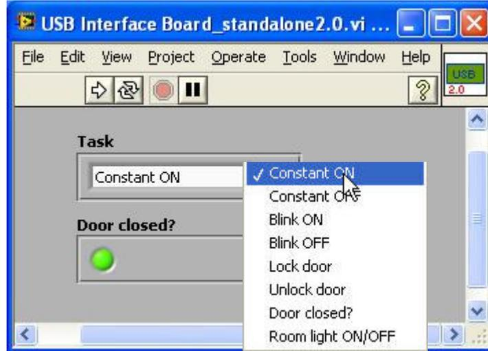
Figure 4-22: Front panel of the *USB Interface Board\_standalone2.0.vi*
