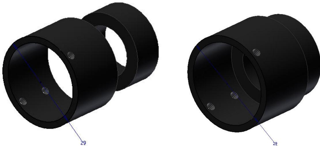
Figure I-10: CAD model of the two rings that keep the photodiode attached to the integrating sphere. (Part IV in figure 4-5)
