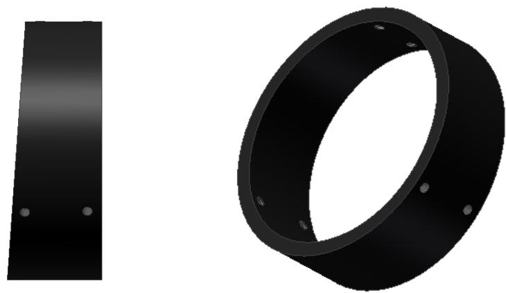
Figure I-11: CAD model of the flange between integrating sphere and monochromator.
