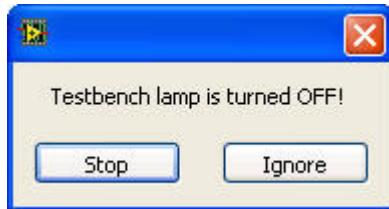
Figure 4-27: Appearin dialog box if the test bench halogen lamp is turned off
