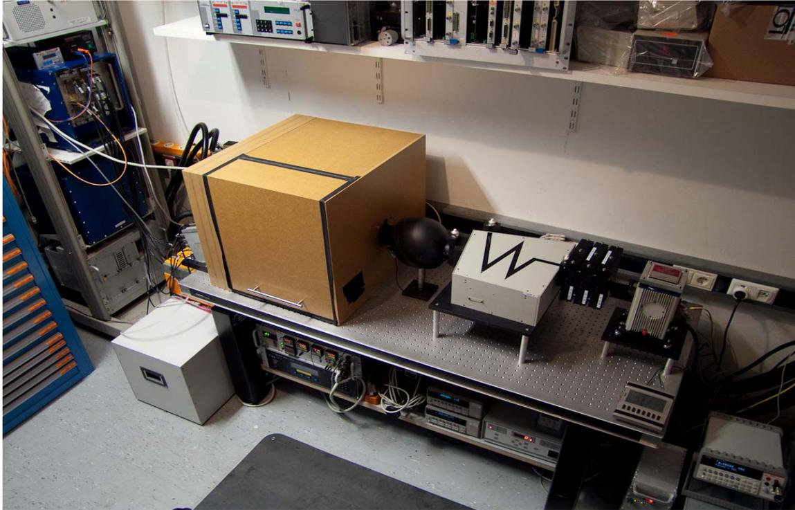
Figure 4-3: The new CCD test bench
