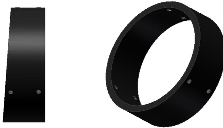
Figure I-11: CAD model of the flange between integrating sphere and monochromator. (Part II in figure 4-5)
