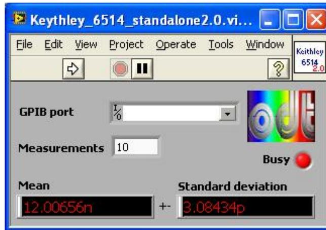
Figure 4-14: Front panel of the *Keythley\_6514\_standalone2.0.vi*
