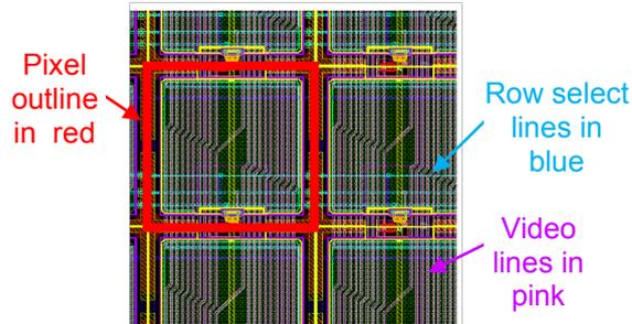
Figure 4-2 : Layout of the pixel showing the three pixel select lines (reset, select and transfer) and the 20 long video lines that run the length of chip up and down from the center lines.
