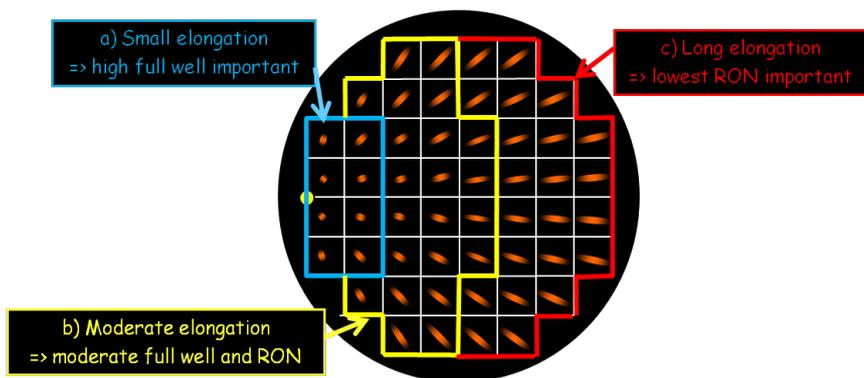
Figure 2-2 : Shows why 9-bit resolution ADCs combined with regions that can be programmed with different gains is an acceptable compromise. Image shows a typical spot elongation pattern for side projected laser. Three different regions are identified: a) region of small elongation where detecting high signal is important, b) region of moderate elongation where moderate signal detector limit and read noise are acceptable, c) region of long elongation where lowest read noise (RON) is important.
