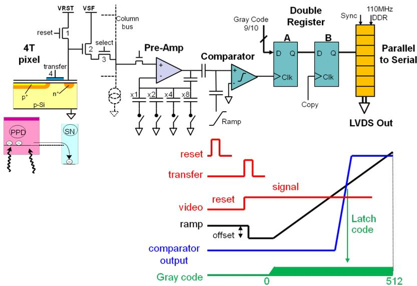
Figure 4-3 : Details of the video processing chain showing pixel, programmable gain pre-amp, single slope ADC (consisting of comparator, Register A, Gray Code counter, and ramp generator), shadow Register B, and serializer (parallel to serial converter).
