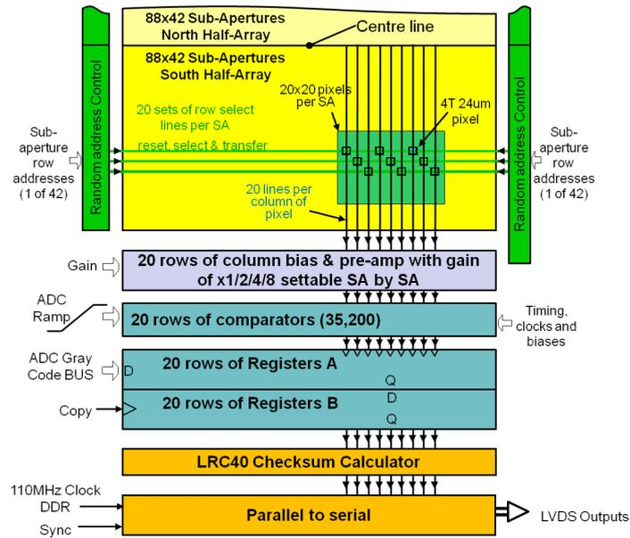
Figure 4-1 : Block diagram of the layout of the read out of NGSD/LGSD.
