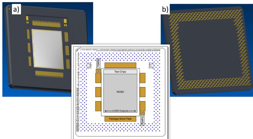
Figure 4-4 : Model of the custom 63 mm square Aluminum Nitride (AlN), 370pin PGA NGSD package, a) front and b) rear view.
