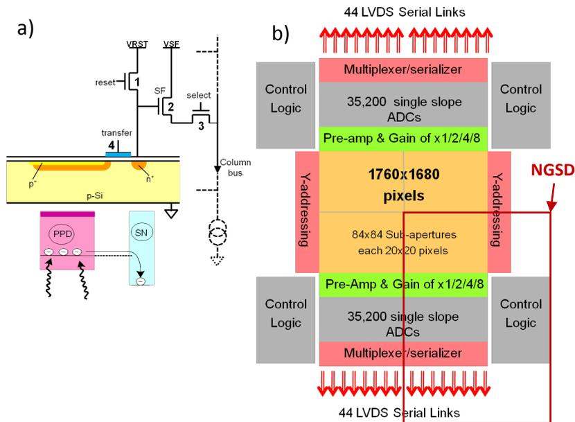
Figure 2-1 : NGSD/LGSD CMOS imager: (a) 4T PPD charge coupled pixels, (b) e2v's conceptual block diagram of the LGSD built using BSI CMOS Imager. The outline of the quarter sized NGSD scaled down demonstrator is shown in red.
