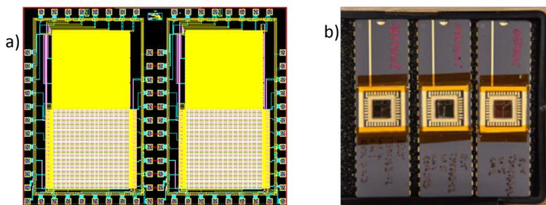
Figure 3-1 : The Technology Validator built by e2v technologies: (a) chip mask layout, (b) Photograph of devices tested. The device featured 60x60 4T pixels, 1200 (60 x 20 rows read in parallel) single slope ADCs, and a read out speed that is consistent with a frame rate of 700fps in the final device.
