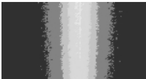
Figure 4-1. Part of a bias at 50kpix/s, binning 15x15, 6ADU of difference between the center and the sides, gain= 0.55e-/ADU
