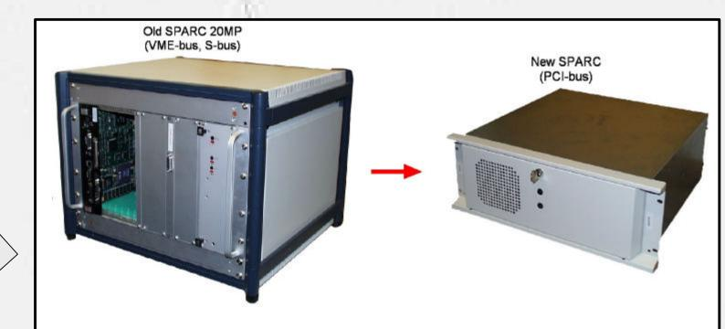
• Higher data throughput: 132MB/s against 40MB/s (S-Bus) • Significant SLCU cost reduction. Factor of five • System more compact. Volume reduction of 30% • PCI: Platform independent • Array of Detector Electronics with one SLCU • Less cabling. Improved reliability
