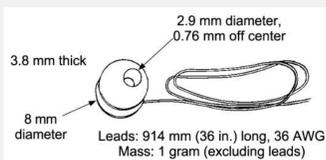
PT100 are a widely used industry standard but suffer from a limited low temperature range. Cernox RTDs have an excellent performance at low temperature (sensitivity) and they work down to ~1K. The chosen type (CX-1080-CU-HT-20L) has an electrical resistance range of approx. 150Ω..8kΩ between 300K and 20K.
