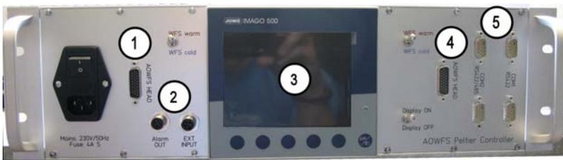
**Figure 20:** Front panel of the Peltier controller. 1) Output for the first camera head. 2) Alarm output and external input connectors. 3) JUMO Imago 500 controller. 4) Output for the second camera head. 5) Serial communication and maintenance connectors.
