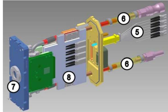
**Figure 4:** AOWFS camera showing 5) Fiber feed-through, 6) Water cooling pipes, 7) CCD window, 8) Rear side of Main board.
