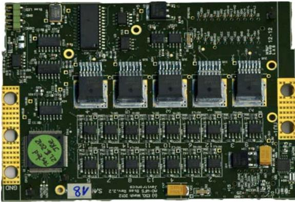
**Figure 7:** Bias board top. As on the Main board the left and right thermal pads are connected to the cooling pipes.
