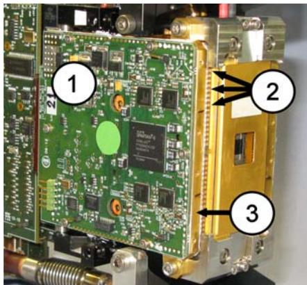
**Figure 13:** AD board and Clock driver assembly. 1) AD board, 2) Contacts on the Clock board, 3) Copper frame thermally connected to the cooling block.
