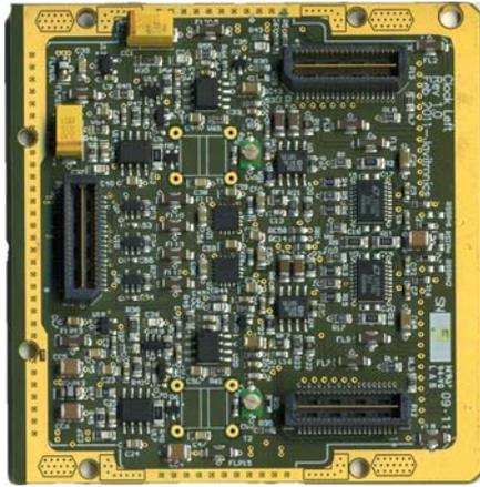
**Figure 11:** Clock board top. The three connectors interface this board to the AD board.
