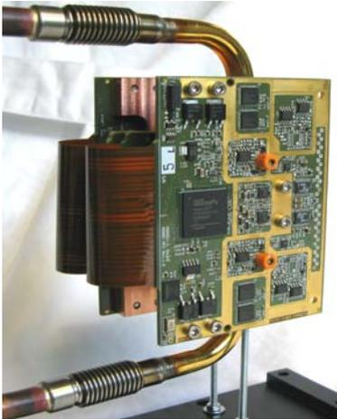
**Figure 15:** Front-end reshaped board combining the old AD and Clock boards.
