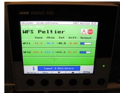
**Figure 21:** Peltier controller display screen.
