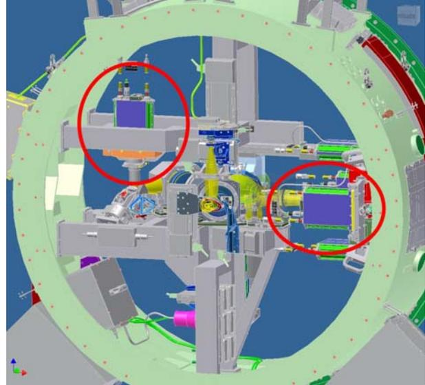
**Figure 28:** GALACSI with two of the four AO cameras highlighted. (Tip/tilt camera not visible)
