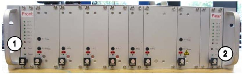
**Figure 19:** Rear side of the power supply showing the voltage supervisors on either side, one for the front set of power supplies (1), and the other for the rear set (2).
