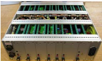
**Figure 18:** Front side of the power supply showing the two MIL circular output connectors on the left side.
