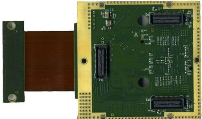
**Figure 10:** AD board bottom. The three connectors on the bottom side interface with the clock driver board.
