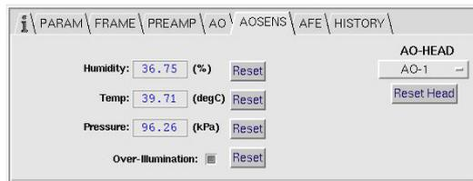
**Figure 17:** Environmental sensors panel. This panel also contains the over-illumination indicator.
