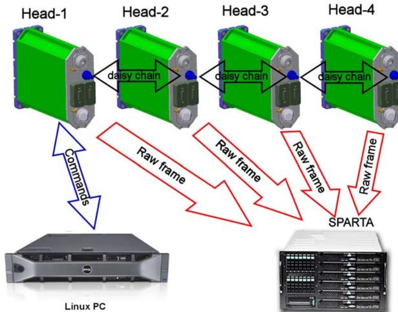
Figure 2: Multi-head connection architecture.
