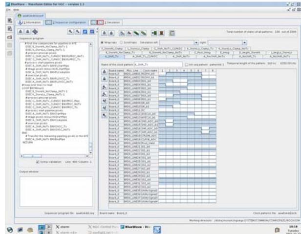
Figure 23: Bluewave, a sequencer and clock pattern programming software.
