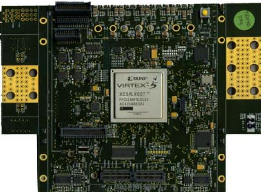
**Figure 5:** AONGC Main board top. The big thermal pads connect the PCB to the thermal cooling pipes via copper clamps.
