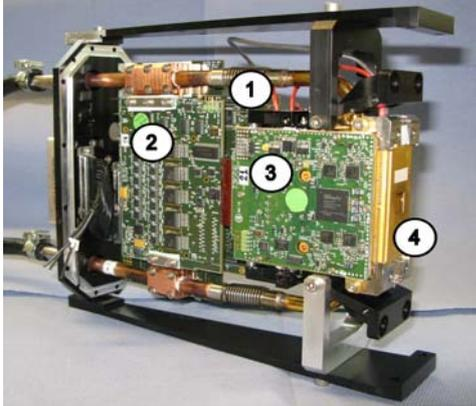
**Figure 3:** AOWFS camera showing 1) Main board, 2) Bias board, 3) AD board left, 4) CCD220.
