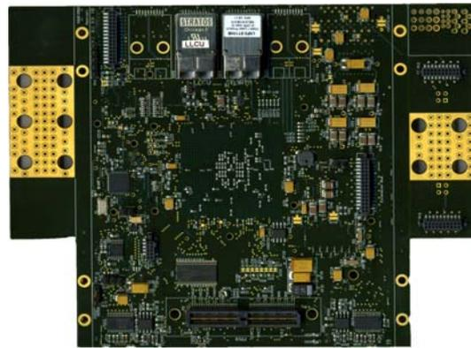
**Figure 6:** AONGC Main board bottom. On the upper side of the board one can see the low-profile optical transceivers LNP-LT12HB (1320nm) and LNP2-ST11HB (850nm), see reference [6].
