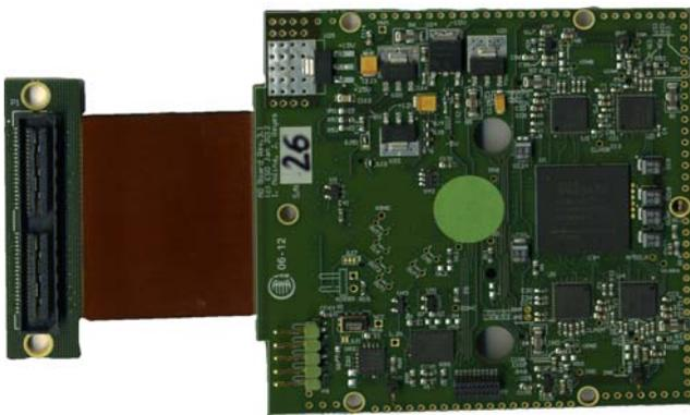
**Figure 9:** AD board top. The board is connected to the Main board via a flex PCB.
