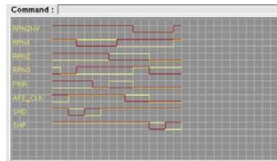
Figure 25: CCD phase programmed and actual phase on the CCD chip after taking into account the delay.
