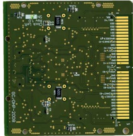
**Figure 12:** Clock board bottom. On the left side one can see the pads for the spring contacts that connect to the CCD.
