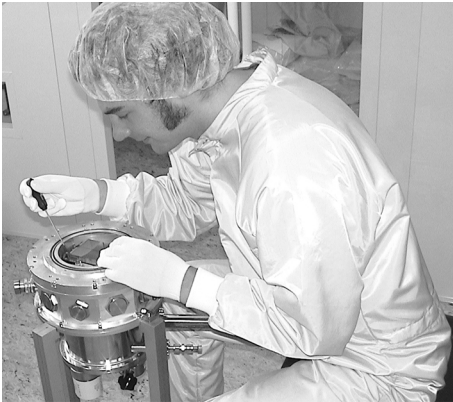
Figure 4: Cryostat assembly in clean-room
