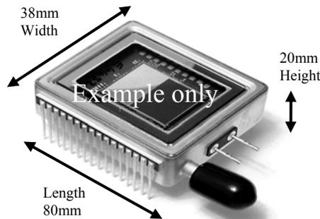
Fig. 11. Photograph of CCD65 Peltier cooling package. The AO CCD220 detector will use a similar Peltier package. Dimensions shown are the requirements on the maximum package size.
