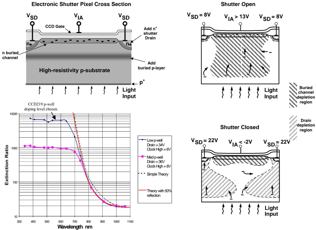
Fig. 6. Principle of the Integral Shutter of CCD219 (see text for explanation). Top left: Cross-section of pixel showing added p-layer implant and  $n^+$  doping to form the shutter drain. Top right: Clock voltages for shutter open. Bottom right: Clock voltages for shutter closed. Bottom left: Expected extinction ratio versus wavelength.
