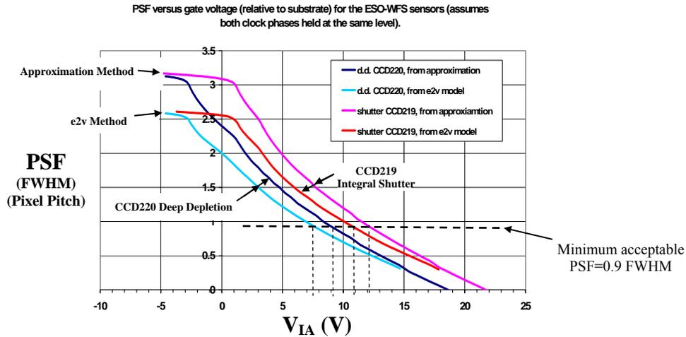
Fig. 7. Simulation of PSF versus image area clock voltage,  $V_{IA}$ , relative to the substrate for the CCD220 deep depleted and CCD219 shuttered devices at worse case wavelength of 460 nm. PSF was predicted by two methods; approximation to the undepleted thickness and e2v model. The dashed line shows the minimum acceptable PSF of 0.9 pixels.
