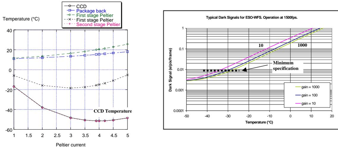
Fig. 12. Results of thermal and dark current modelling. Left: Predicted temperature of the CCD versus Peltier current modelled by Philippe Feautrier<sup>9</sup>. Right: Dark current versus temperature modelled by e2v for the baseline standard silicon CCD220 when the image area is operated fully inverted.
