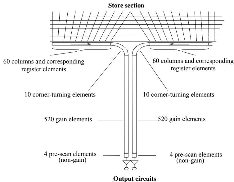
Fig. 3. Details of serial and gain register.
