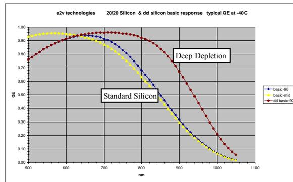
Fig. 5. Comparison of QE for a standard silicon device (basic-90/basic-mid) to that of a deep depletion device (dd basic-90). These curves are only typical and the curves of the final devices may differ.
