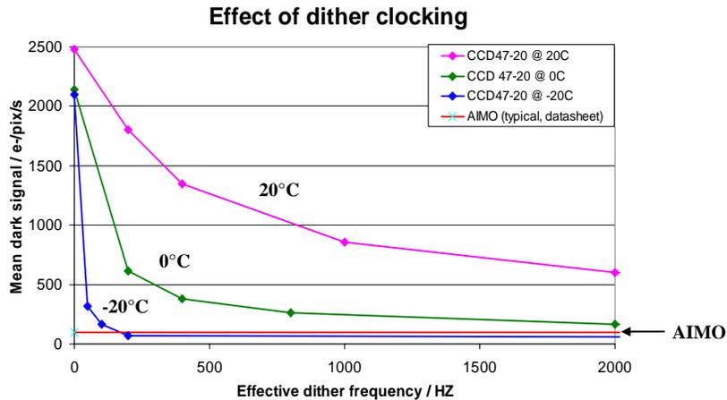
Fig. 8. Results of measurement performed at e2v on a CCD47-20 at various temperatures to demonstrate “intrinsic dither mode”. The curves have been scaled differently for convenient plotting. The main item to note is that at the lowest operating temperature (-20°C) the dark current reduces at high readout rates. This process is expected to apply to the CCD220 at operating temperature of -40°C.
