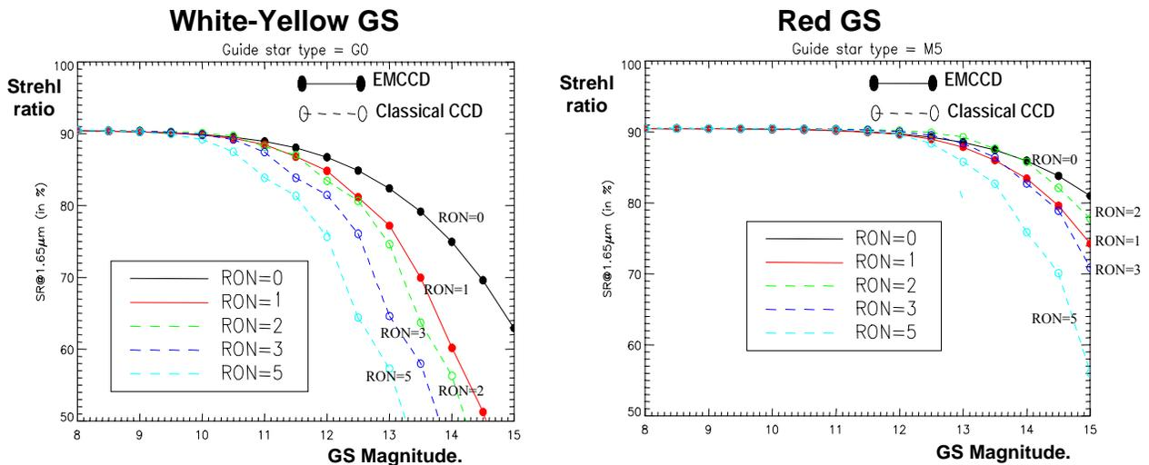
Fig. 1. Results of analysis performed by Thierry Fusco for ESO instrument SPHERE that compares an EMCCD of read out noise (RON) 0 and 1e- to a classical CCD of read noise 2, 3, and 5e- for two different types of guide stars. Left: Plots of Strehl Ratio versus GS magnitude for white-yellow guide star. Right: Plots of Strehl Ratio versus GS magnitude for red guide star.
