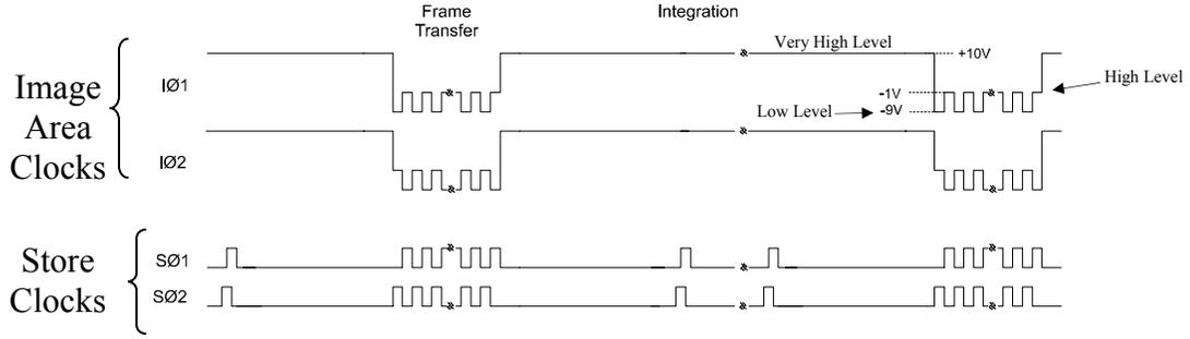
Fig. 9. Example clocking scheme for the deep depleted CCD220 using tri-state image area clocks. This mode should minimize the dark signal and CIC while maximizing the PSF performance.
