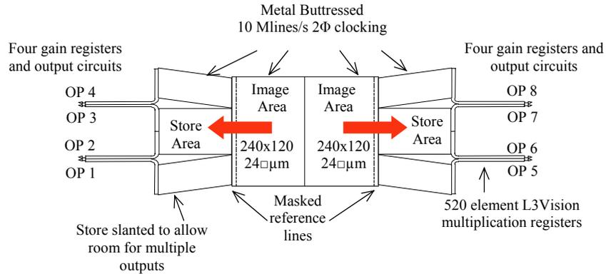
Fig. 2. Schematic of CCD220.
