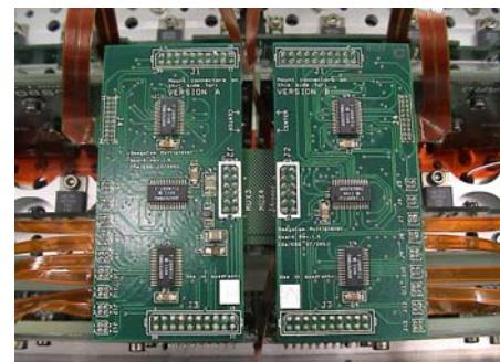
Figure 23: CCD head integrated dual multiplexer
