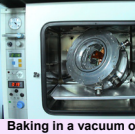
Baking in a vacuum oven
