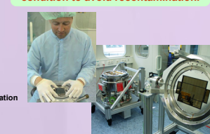
OmegaCam cryostat inside the clean-room
