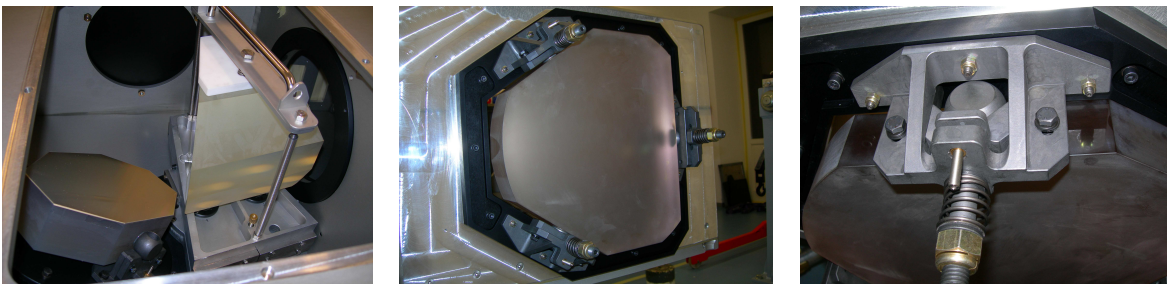
Figure 8: Mechanical mounts of the prism-grating unit, the main collimator mirror, and details of one of the mirror supports.
