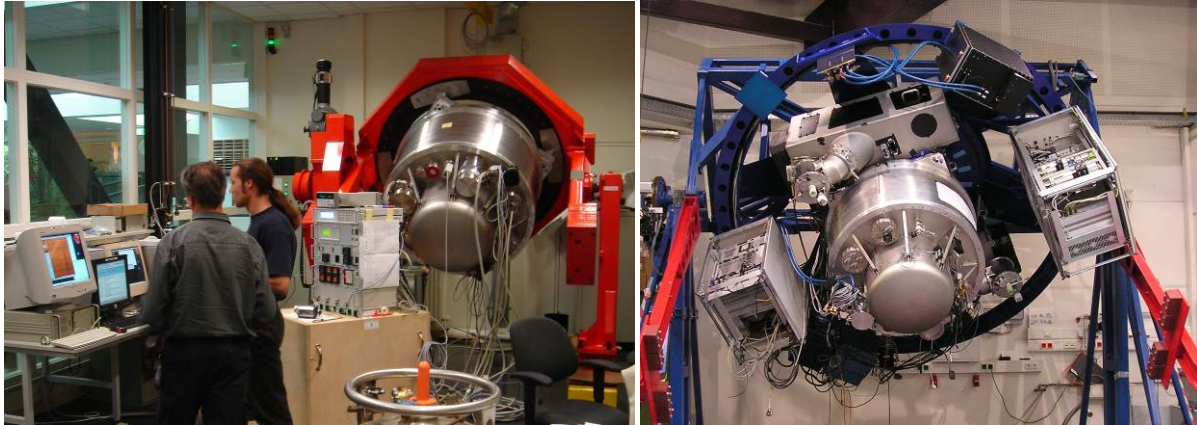
Figure 13. X-shooter near infrared spectrograph during tests at NOVA-ASTRON (left image). The cryostat is mounted on a dummy backbone that is mounted on the telescope simulator (right). The Cold Optical Box is located inside the cryostat. Other equipment comprise the cryogenic control electronics (center) and 3 workstations to control the detector, run the VLT software and analyze all data. The top of one of six liquid nitrogen tanks is visible in the front. X-shooter integrated with the backbone, UVB and VIS spectrographs and electronics in the ESO lab (right image).
