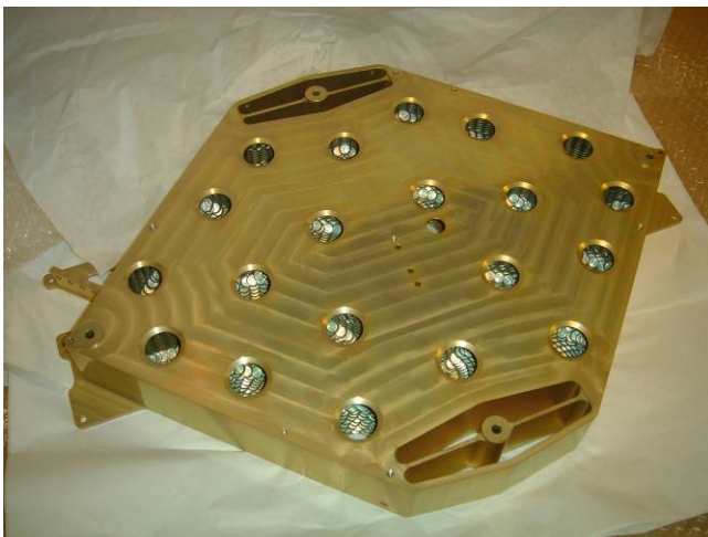
Figure 4. Balance Arm using the ASTRON extreme light-weighting technique. Large internal volumes (pockets) are created by milling through small entrance holes. The weight of the 540 \times 400 \times 57 \text{ mm} aluminium balance arm is 2\text{kg} , which corresponds to lightweighting percentage of 90\% . Internal ribs in the pockets improve the overall stiffness.
