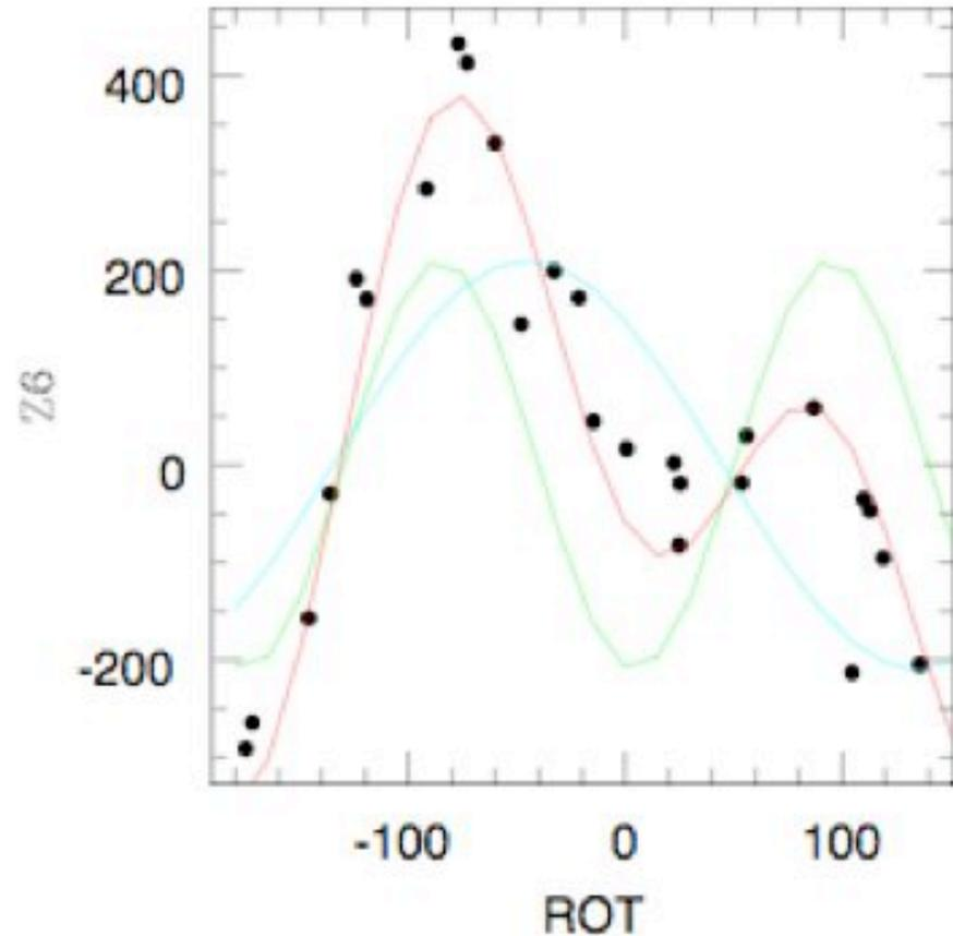
2 component model with a true field corrector misalignment term and a 'phantom' 2-theta term from the gradient of the M1 trefoil correction
