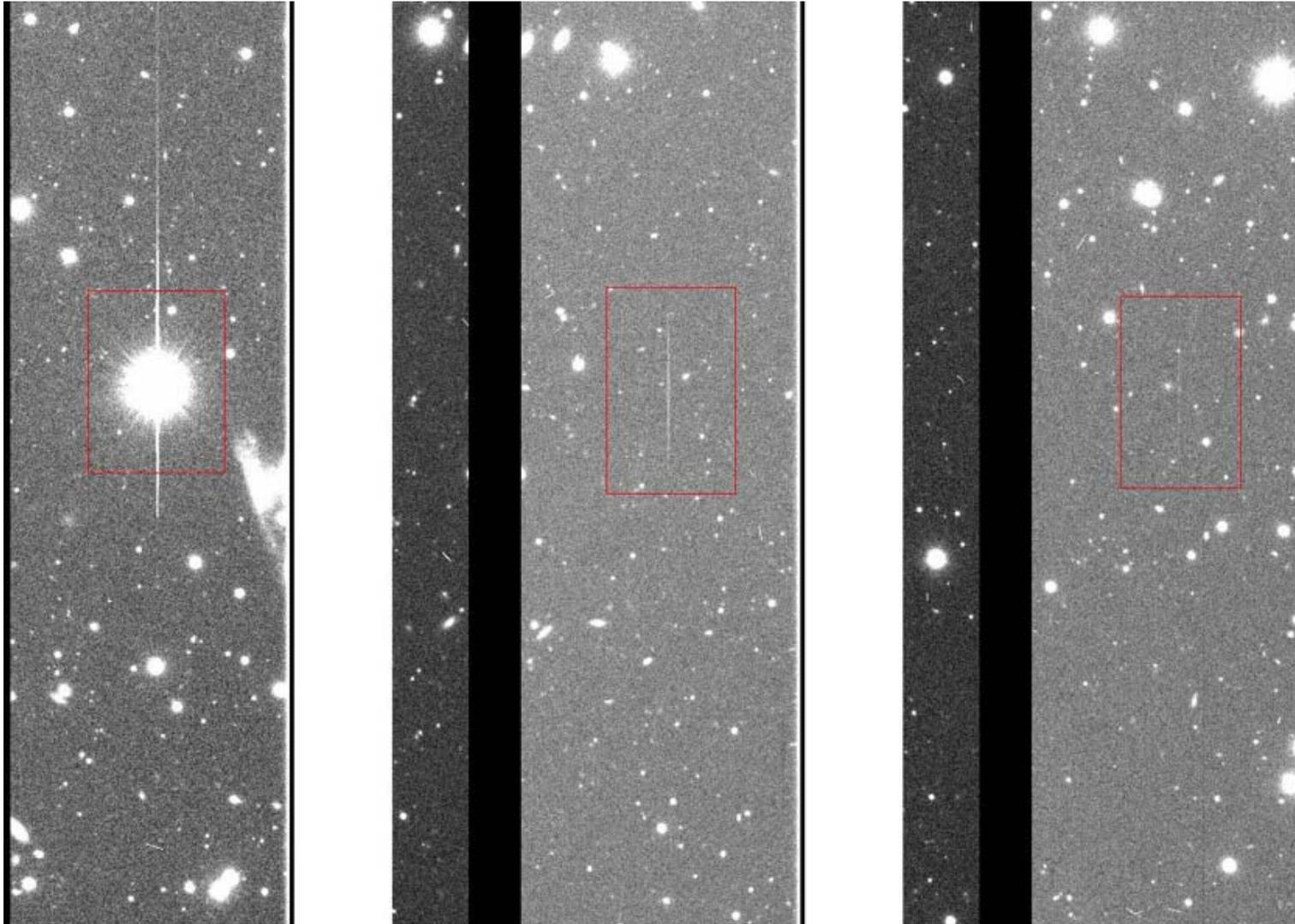
Delayed charge emission from the surface traps
