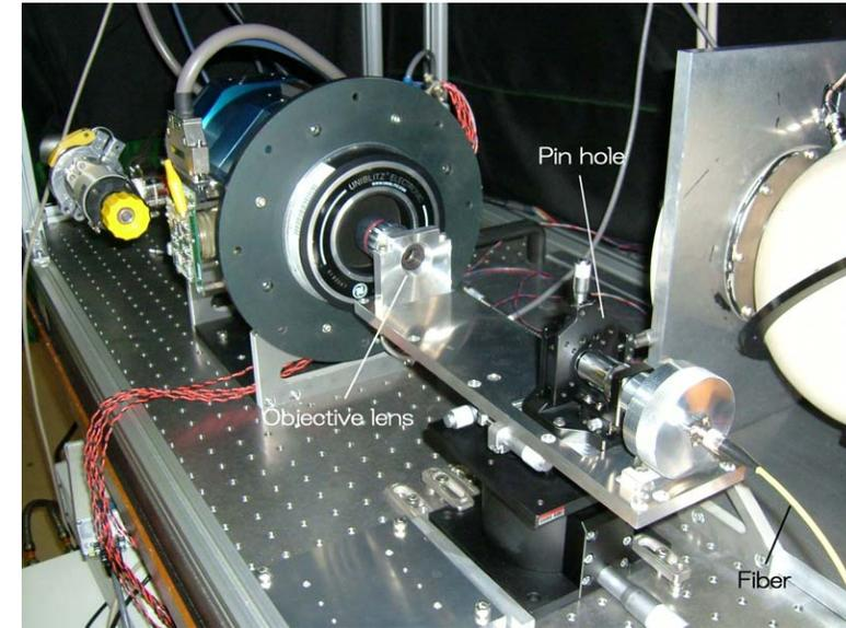
10 micron pin hole is projected with X 1/10 (NA ~ 0.25) optics
