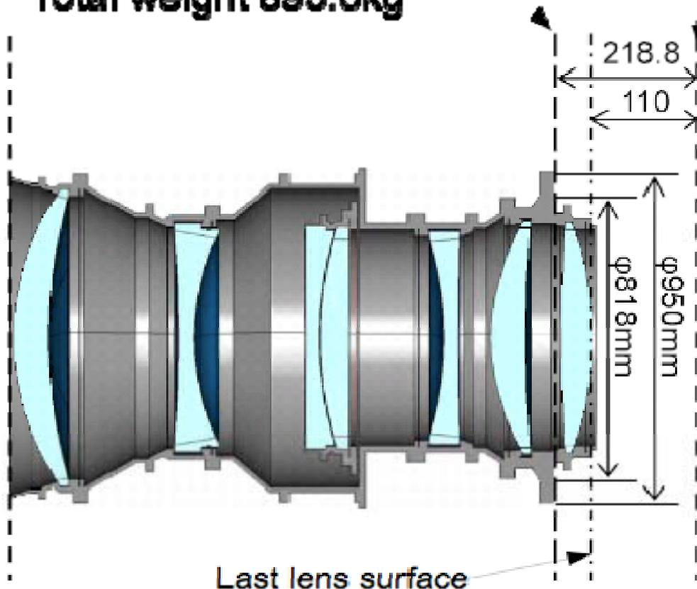
**Each Lens Element is retained by each lens frame.**
