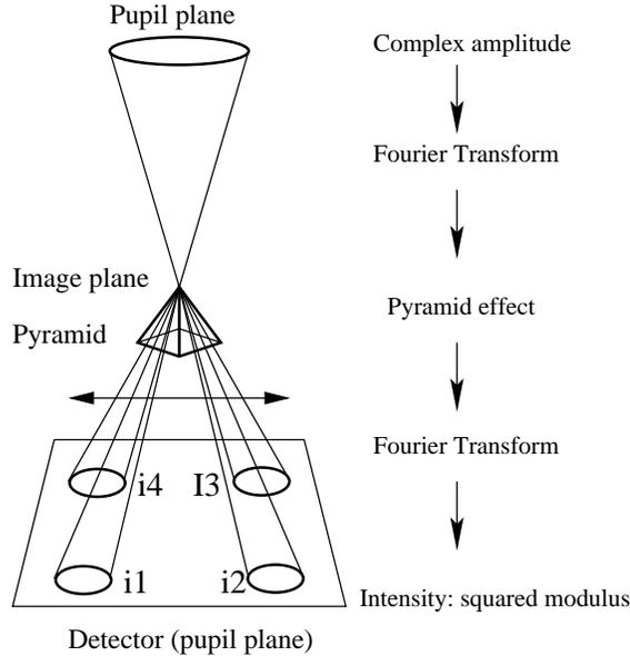
Figure 1. Main steps for the pyramid sensor simulations
