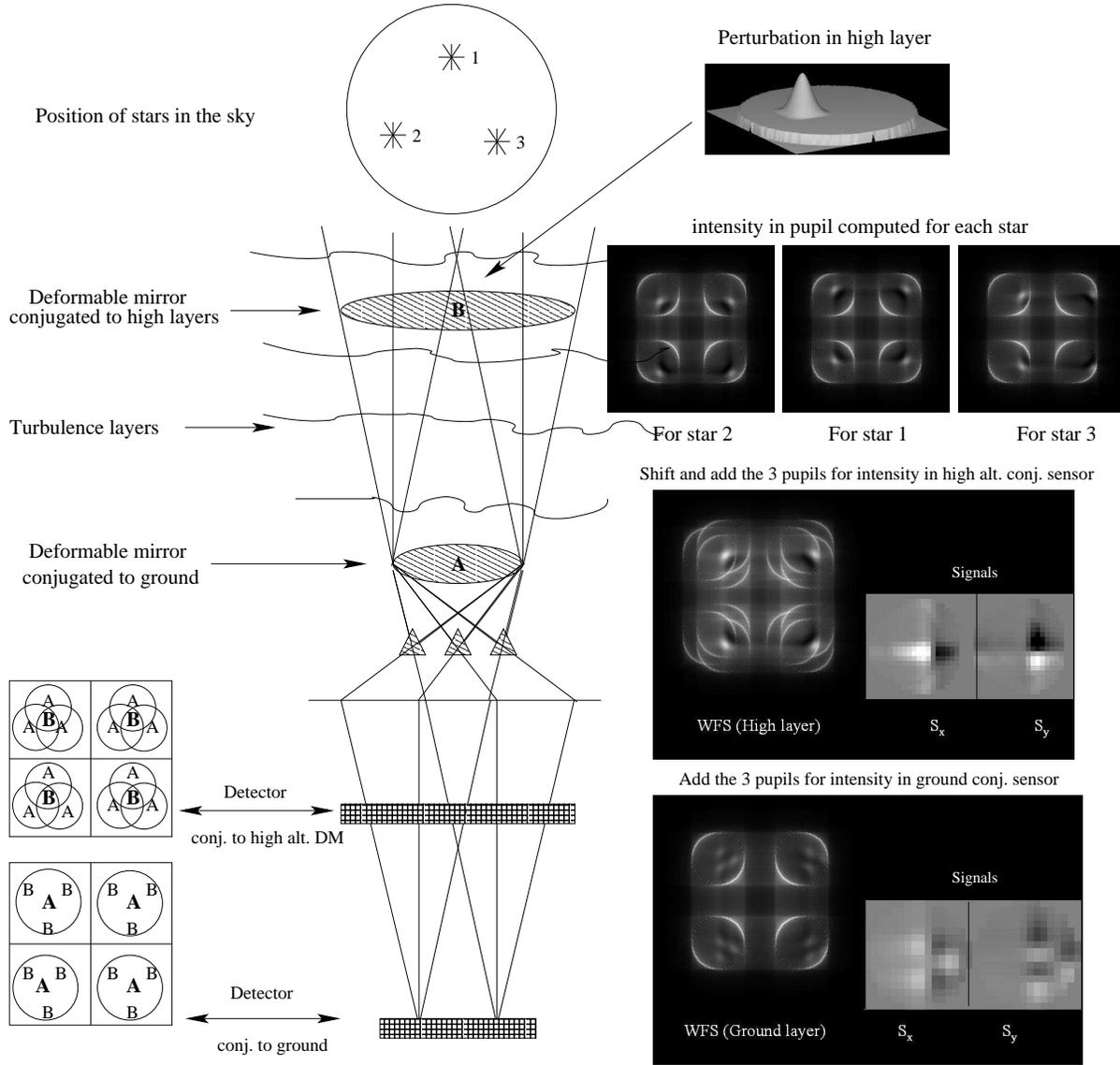
Figure 2. The Layer-Oriented wave-front sensing concept based on refractive Pyramids and method for simulation.
