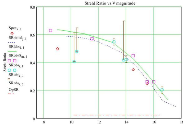
Figure 3. Comparison between the performance of MACAO in simulations and on the sky. Strehl ratio (K-band) vs. guide star magnitude. The top line is the curve obtained in the lab, the dashed line is the simulation, squares and circles are results obtained at the telescope, diamonds are the specifications, the dot-dashed line is the open loop seeing. Courtesy R. Arsenault and the MACAO team.
