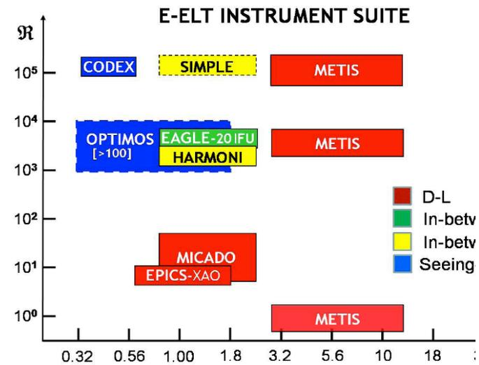
Figure 4: Spectral resolution ( $R$ ) - wavelength ( $\lambda$ ) chart for the current E-ELT instrument suite (conceptual studies). Colour-Coded and (Diffraction Limited) yellow
