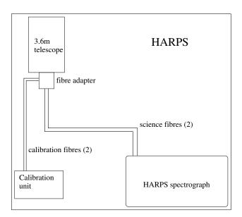
Figure 2.4: The main components of the HARPS system
