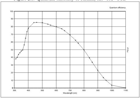
Figure 2.6: Quantum efficiency of Linda, the "blue" CCD
