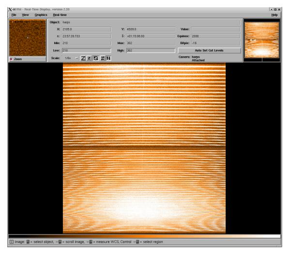
Figure 6.2: The Real Time Display of a HARPS spectrum taken with the tungsten lamp illuminating both fibers. The lower part is the blue chip ("Linda"), the upper one is the red chip ("Jasmin"). Wavelength increases from lower left to upper right.
