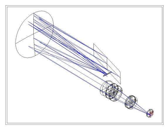
Figure 2.1: Optical layout of the spectrograph
