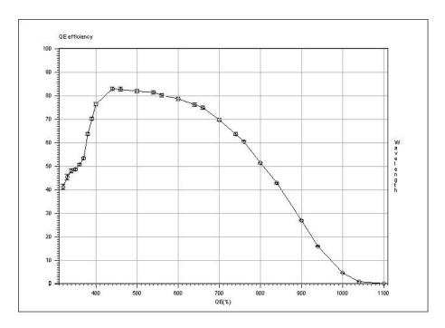
Figure 2.5: Quantum efficiency of Jasmin, the "red" CCD
