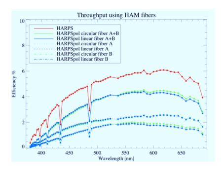
Figure 3.1: Throughput of HARPS with and without the polarimeter, for both the linear and the circular polarimeter.
