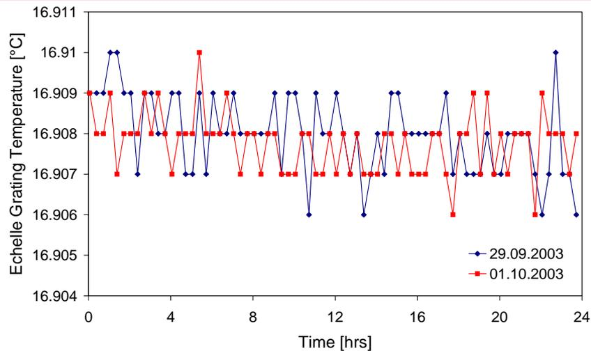
**Figure 1.** Temperature of the spectrograph echelle grating during 24 hours and at two different days. The stability during one day is of the order of 0.001 K *rms* while the yearly stability is better than 0.01 K
