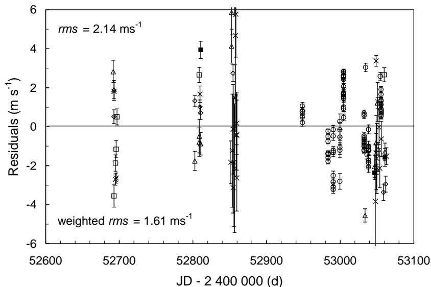
**Figure 6.** Plot of the residuals of many different stars (different symbols) from our planet search survey sample since the “First Light” of HARPS. The “all included” *weighted rms* is  $1.6 \text{ ms}^{-1}$ , despite the fact that several critical instrument changes have been carried out between first light and the start of operations in October 2003. The error bars indicate the pure photon noise level and therefore do not take into account external errors such as stellar contributions.
