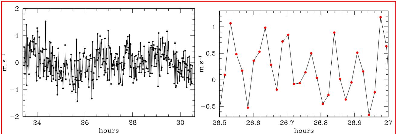
**Figure 3.** a) Series of 7 hours and 420 exposures on  $\alpha$  Centauri B proving the extra-ordinary short-term precision of HARPS. b) Zoom into part a) to illustrate the presence of a periodic signal produced by the star's pulsation.
