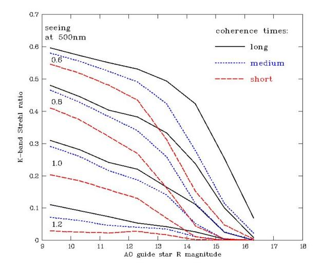
Figure 1: The predicted Strehl performance in K band is shown on the following figure for some seeing cases (0.6 to 1.2" at 500 nm) and high altitude wind speeds of 11 m/s (long), 22 m/s (medium) and 33 m/s (short):
