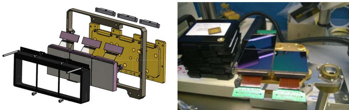
Figure 7: The 3 CRIRES H2RG detectors are shown (right) together with the detector mount (left)
