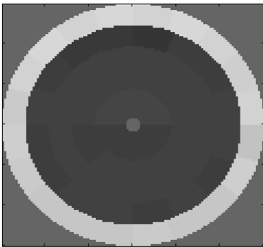
Figure 14: voltage pattern for a piston term. Outer electrodes are submitted to the highest voltages
