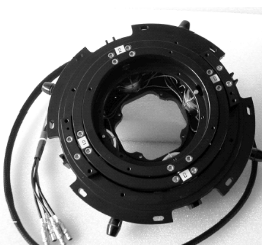
Figure 7: tip-tilt mount, front view; the four linear actuators are visible inside the mount, at 45° from the handles.
