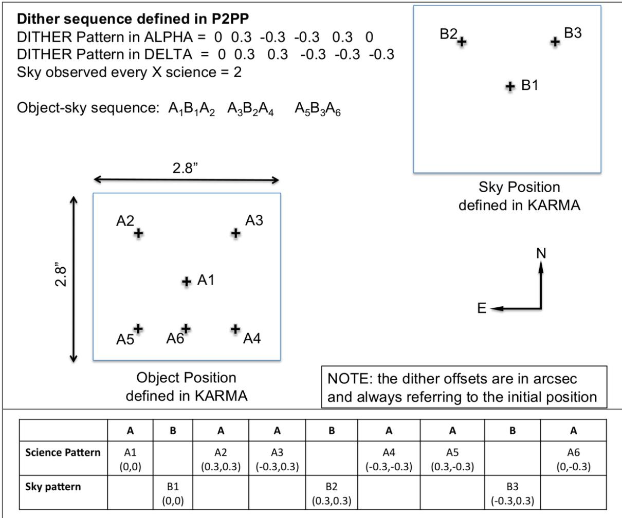
Figure 15: An illustration of the dither pattern that can be constructed with the free-dither template in p2. The sequence for just 1 IFU is shown, since it will be identical for all of them. This example is for 6 object frames and sky frequency = 2, which gives in total 3 sky frames in the sequence ABA ABA ABA.
