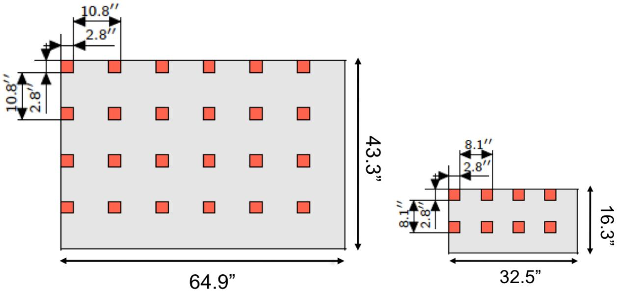
Figure 11: Left: The size of the continuous area ( $\approx 0.8$  sq. arcmin) covered by a single OB in Mosaic mode with the large configuration with 24 IFUs, which requires 16 telescope pointings. The red squares indicate the IFU positions at the start of the OB. Right: The small Mosaic configuration with 8 IFUs, which requires 9 telescope pointings to cover the rectangular area of  $\approx 0.15$  sq. arcmin.
