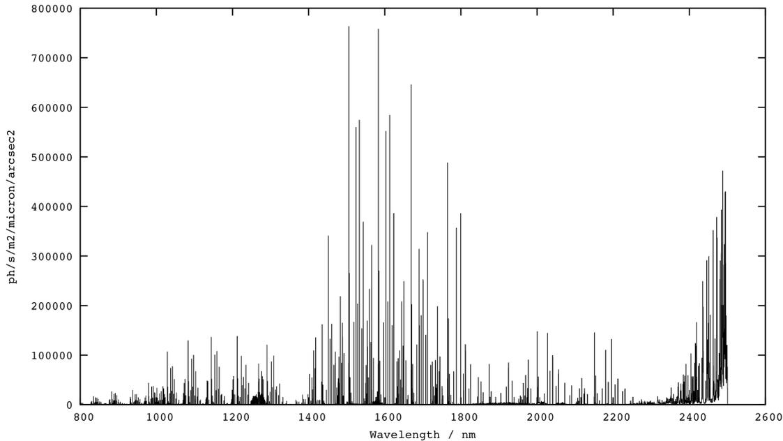
Figure 12: Sky emission as a function of wavelength.
