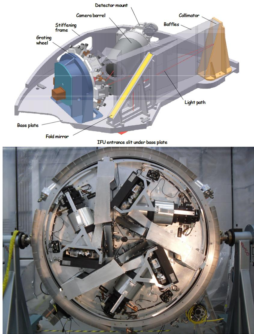
Figure 5: Top: Perspective view of a single KMOS spectrograph module. Bottom: the three spectrographs mounted in the KMOS cryostat.
