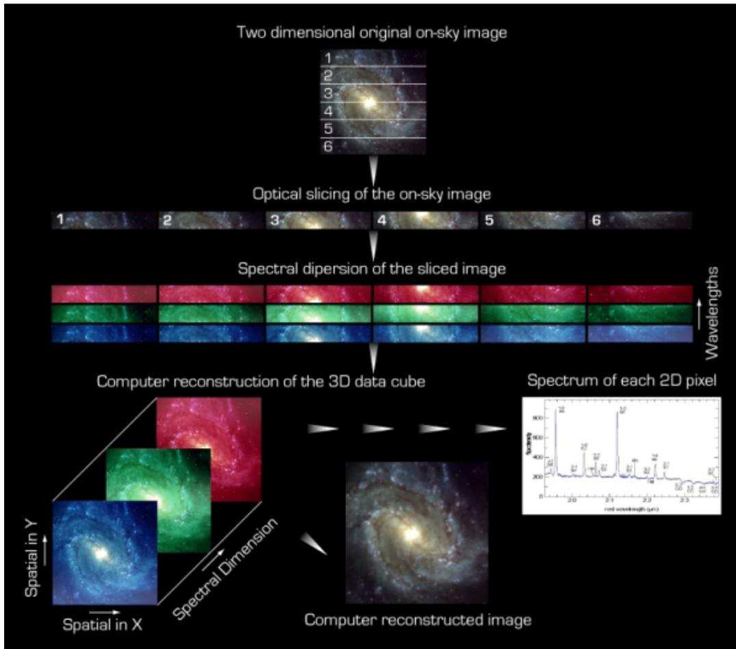
Figure 1: Example of Integral Field Unit Spectroscopy. A 2-dimensional image will first be sliced, the slices then dispersed on a common slit and finally a 3D data cube is reconstructed from the obtained spectra. In KMOS the image is sliced in 14 elements instead of 6 as in this figure.
