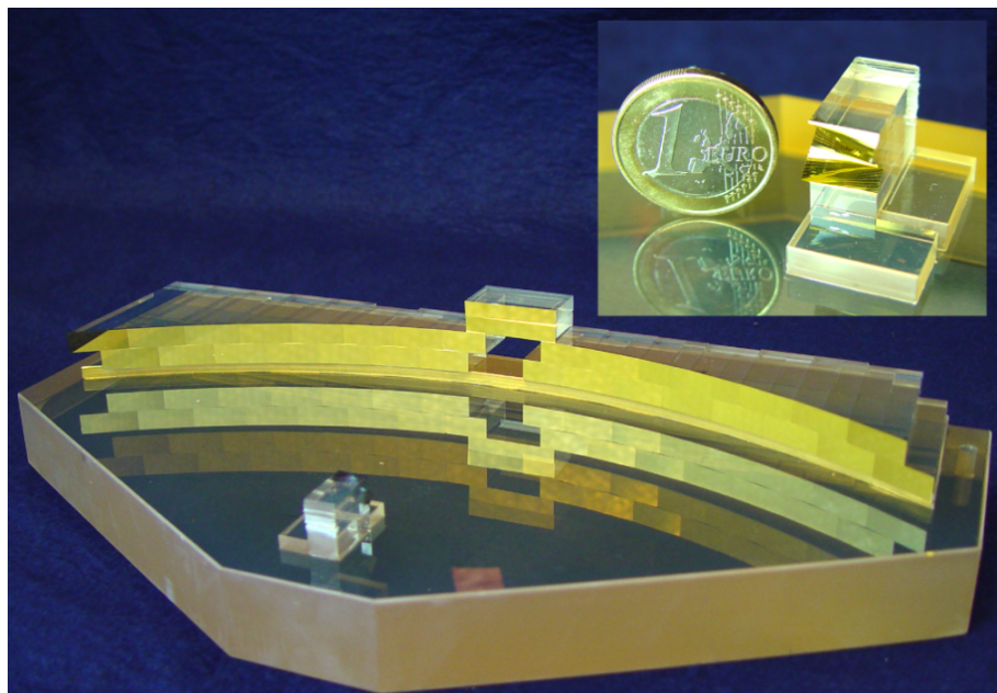
Figure 13: SPIFFI image slicer (a): The light enters through the hole in the big slicer. A stack of 32 small mirrors, the small slicer (also shown in the sub-panel), slices the image and redirects the light towards the 32 mirrors of the big slicer, which re-arranges the slitlets into a 31 cm long pseudo-slit.
